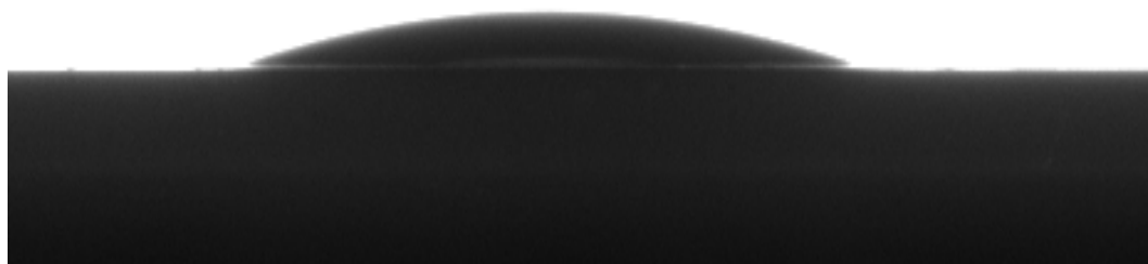
Figure 4.4: Instantaneous droplet shape of C 4 H 4 F 6 O on a plain surface
