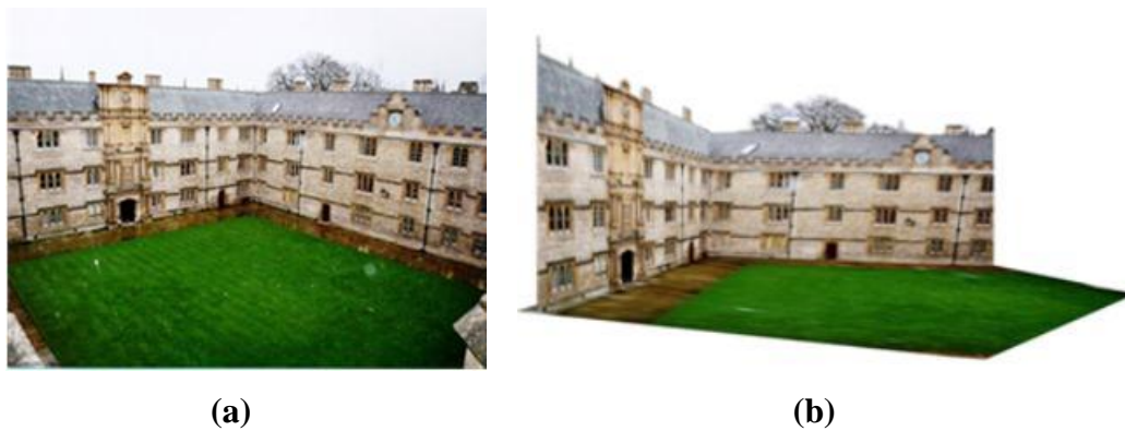
Figure 27. Example output of automatic 3D reconstruction using Hoiem et al.'s approach. (a) Original input image by Liebowitz et al. [51]. (b) Novel 3D view from [44].
