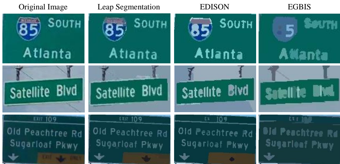
Figure 21. Lettering on street signs is processed using different segmentation approaches for detail preservation comparison.
