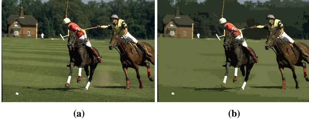
Figure 6. Leap segmentation output example (Polo). (a) Original image 481x321 pixels. (b) Image segmented using leap segmentation (Forsthoefer et al.) [34] with 180 segments.
