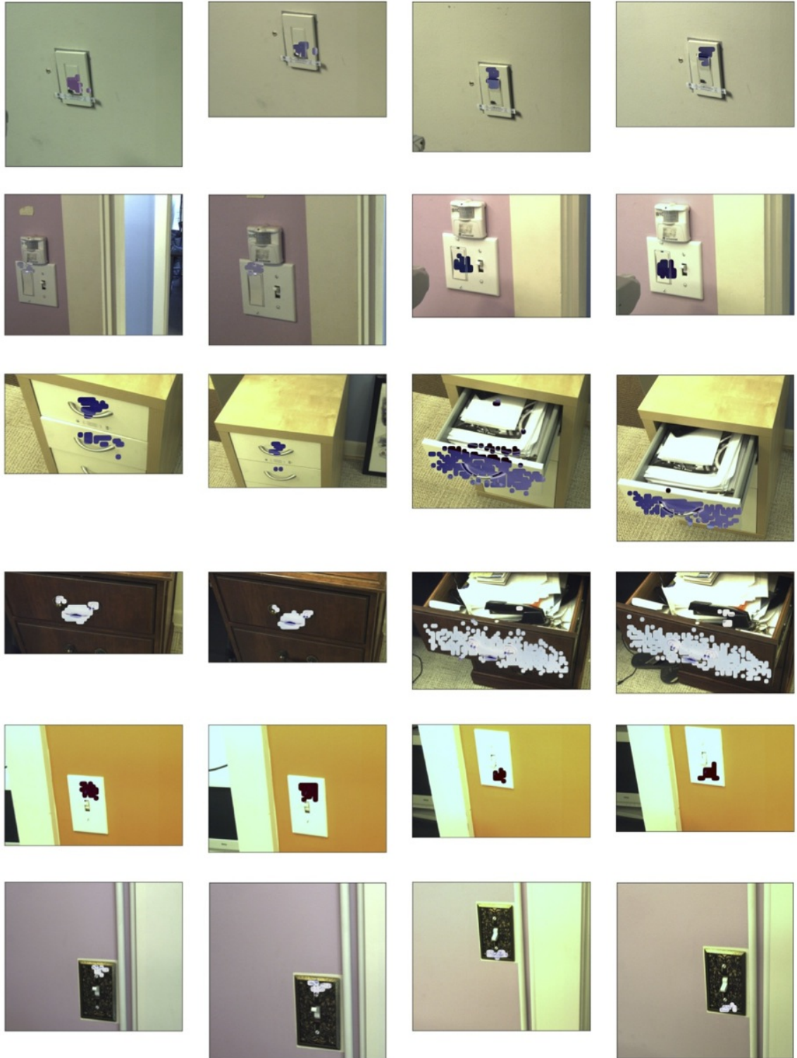
Figure 32: Each pair of images shows classification results of learned detectors just after convergence then on a new test image. Areas with inverted colors mark locations identified as leading to success of associated behaviors. To show these results, we took positively predicted points, placed those points in a grid, then overlaid this grid on the original image. Row 1: Detectors for a rocker switch in our lab. Row 2: Detectors for a different rocker switch in the Aware Home. Row 3: Detectors for pushing and pull a wooden drawer. Row 4: Detectors for another dark wooden drawer. Row 5: Detectors for a regular light switch. Row 6: Detectors for an ornate light switch.
