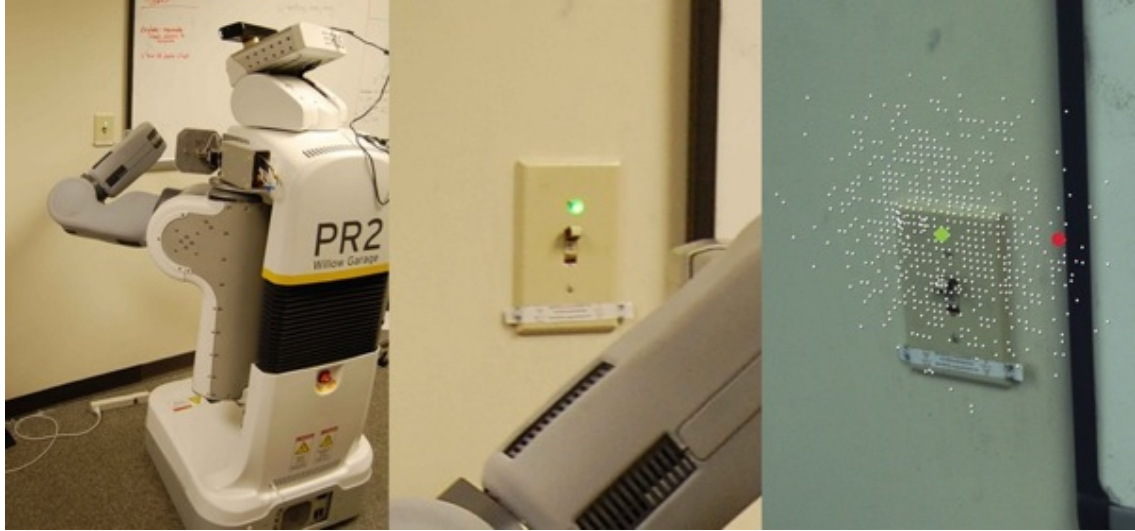
Figure 26: Illustration of the initialization procedure for a pair of behaviors that flip light switches. Left Position robot in front of the switch. Middle Illuminate an initial 3D location as input to the behavior using a laser pointer. Right A 3D location associated with success (green) and a 3D location associated with failure (red) after initialization. Candidate 3D locations to explore are shown in white.
