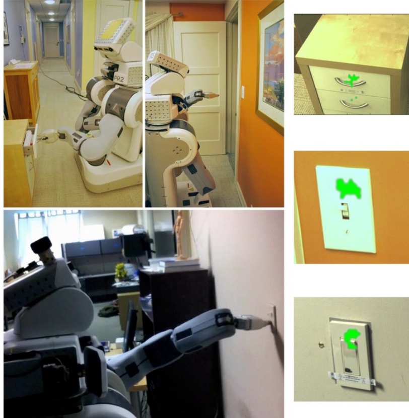
Figure 23: Left: Willow Garage PR2 operating a drawer, light switch and rocker switch using learned detector that detects regions where manipulation will succeed. Right: Results from learned detectors during execution.
