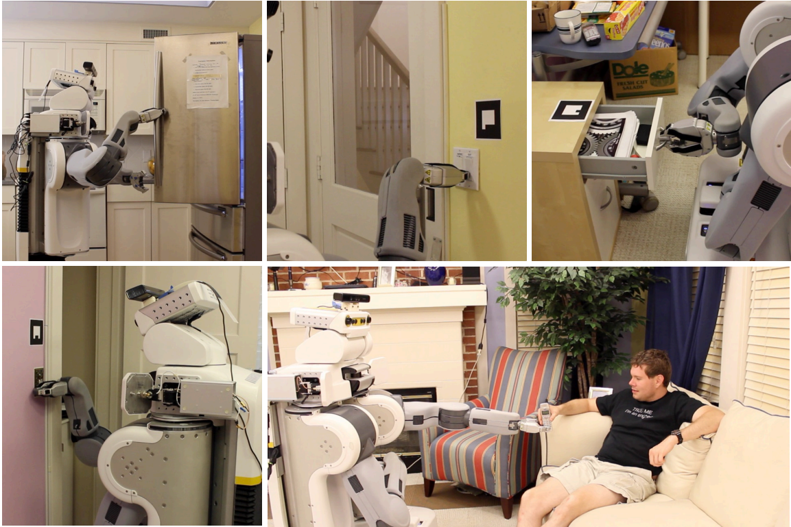
Figure 2: Examples of robot behaviors constructed using the ROS Commander system and encapsulated as HFSSMs: opening a fridge, unlocking with a button, opening a drawer, flipping a light switch, handing off an object.
