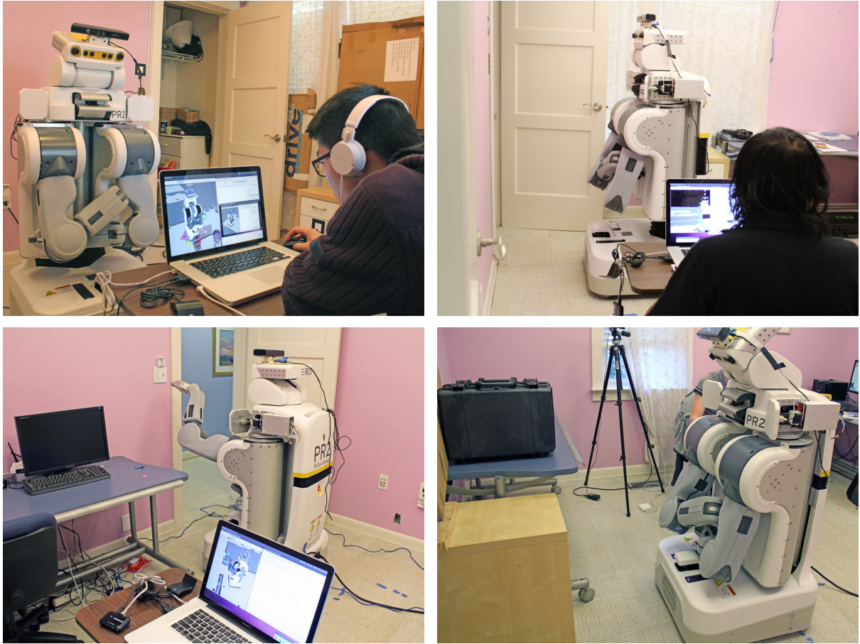
Figure 11: Positioning of robot and participant for each module. Top Left: Subject constructs a waving behaviors. Top Right: Constructing a behavior to turn on the lights with a flip switch. Bottom Left: Participant constructs a behavior that pushes a rocker switch to turn off the lights. Bottom Right: Subject creates a behavior that pulls open a drawer.
