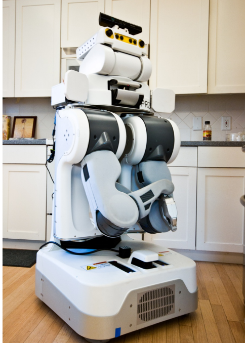
Figure 1: GATSBII, the PR2 used in this work. Photo courtesy of Jerome Choo.
