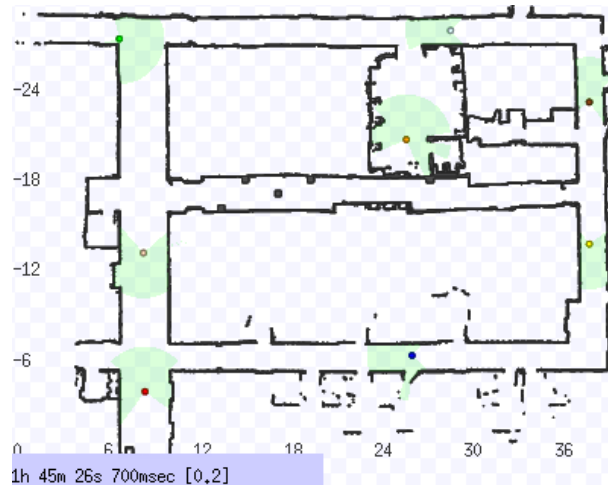
Figure 33: The Stage multi-robot simulator is shown with eight robots patrolling the environment. The robots in the simulation run the ROS navigation stack and participate in auctions for task reassignment.
