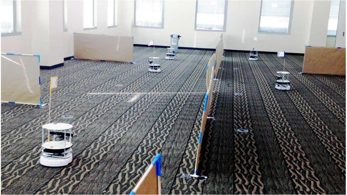
Figure 57: Multiple TurtleBots are shown patrolling in the experimental environment, setup to resemble an art museum with multiple rooms.
