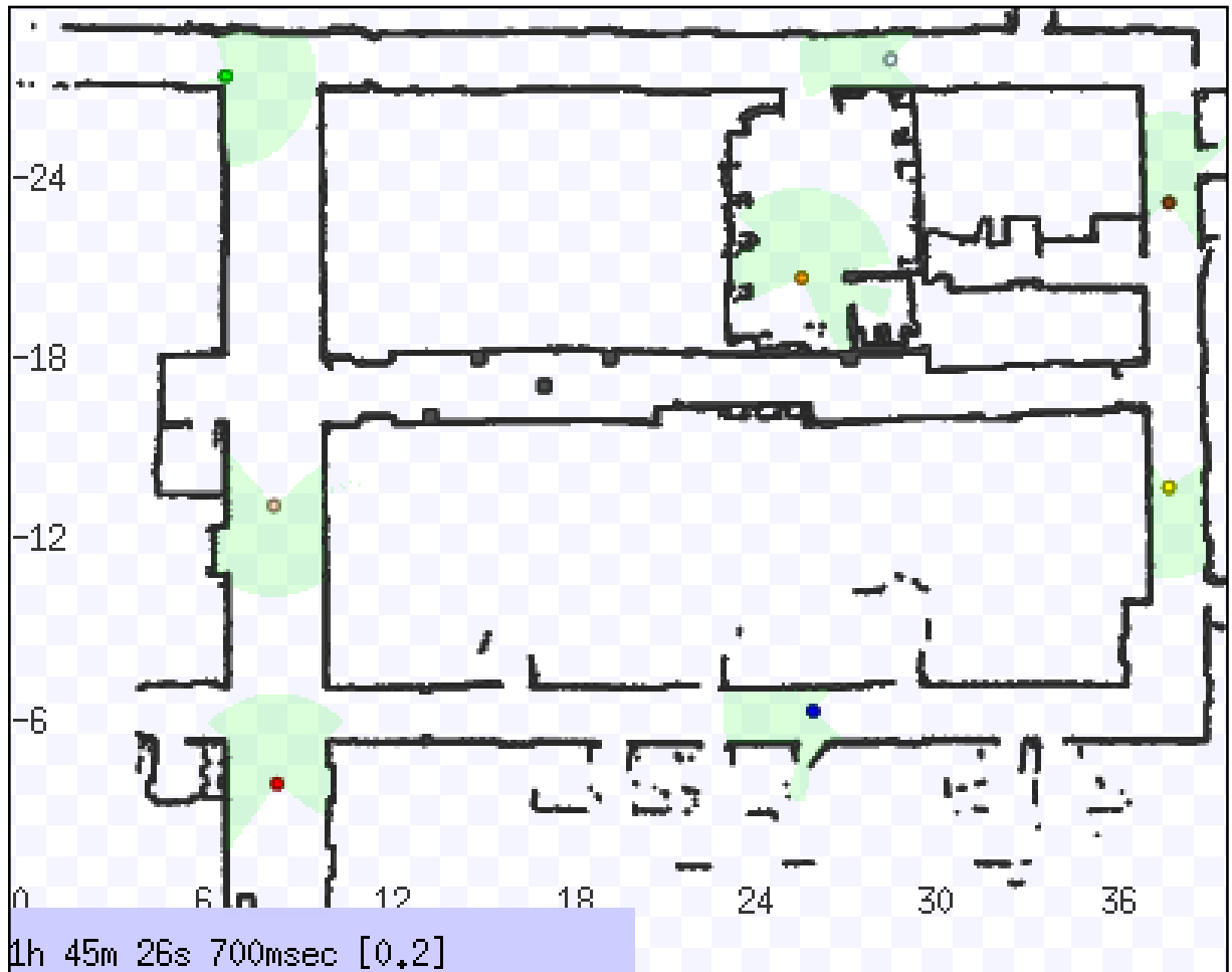
Figure 77: The same autonomous behaviors that run on the real Turtlebots can be tested in simulation. Multiple Turtlebots are shown patrolling in the ROS Stage simulation environment.
