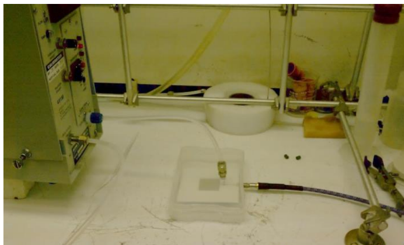
Figure 39. Closed test cell connected to gas generator and PNA.
