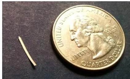
Figure 5.17. The aluminum cantilever is fabricated separately from the 100 \mu\text{m} thick aluminum sheet.
