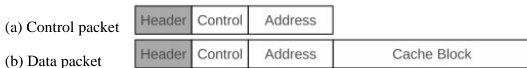
Figure 23: Abstract visualization of the size of the two main packet types generated by the MOESI-CMP-directory implementation of the GEMS simulator [6]. In general, the types of messages traversing the NoC of a CMP are dependent on the employed cache coherence protocol.
