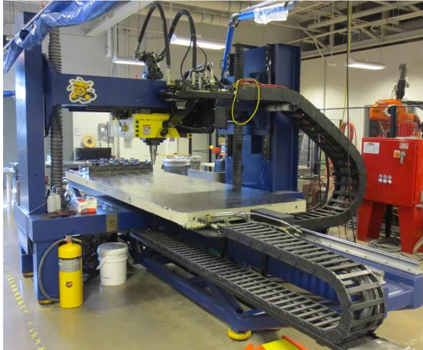
Figure 3.2. Five-axis MTS I-Stir™ PDS machine at Wichita State University.
