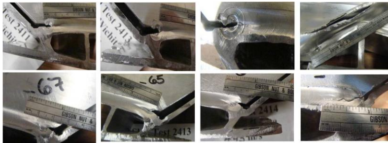
Figure 7.11. Cracks at 7, 10, 15, and 20 kph energies for FSW (columns left to right, respectively).
