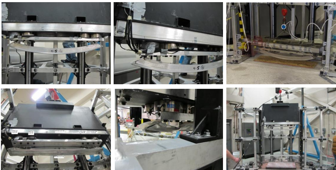
Figure 7.6. Drop tower testing setup.
