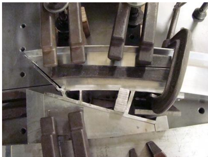
Figure 6.7: Tooling for friction stir butt weld.
