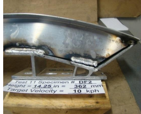
Figure 7.17. Separated corner welds at 10 kph.
