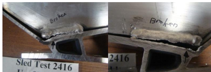
Figure 7.7. Complete separation in GMAW bumpers.
