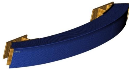
Figure 8.2. Finite element mesh of bumper-beam/crash-box assembly.
