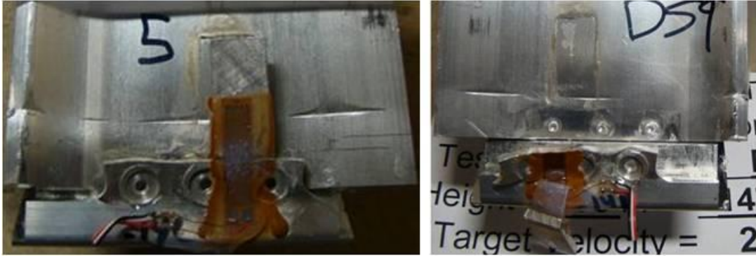
Figure 7.19. Spot separations at 15 kph and 20 kph energies (left to right).
