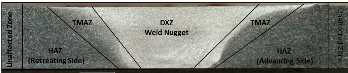
Figure 2.2. Schematic of butt joint cross section showing four distinct zones.
