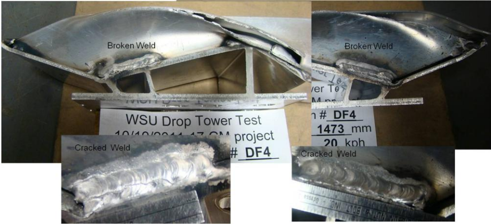
Figure 7.21: Damage in two broken welds and two cracked welds at 20 kph energy.
