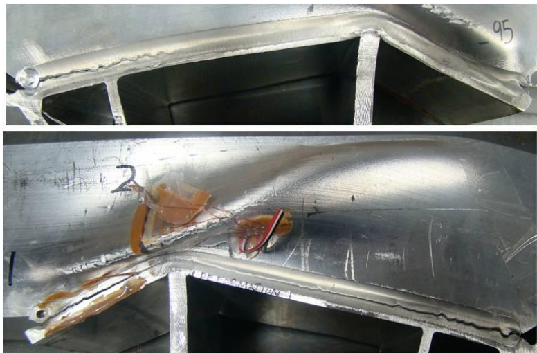
Figure 7.23: FSW cracks and deformation necking under ruptured bumper wall at 15 kph energy
