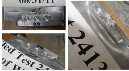
Figure 7.10. Deformation of spot weld at 7 kph (left) and 10 kph (right) energies.
