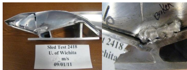
Figure 7.8. Failures in GMAW bumpers.
