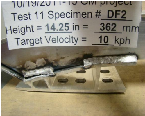
Figure 7.17. Separated corner welds at 10 kph.
