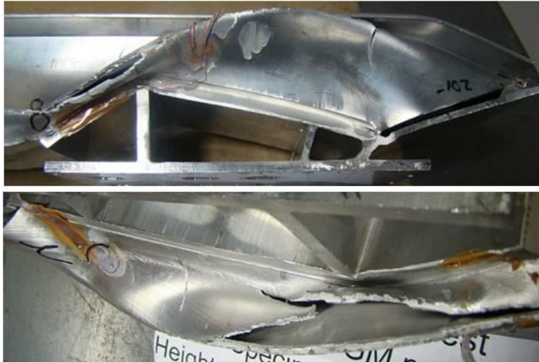
Figure 7.24: FSW cracks under ruptured bumper wall at 20 kph energy.
