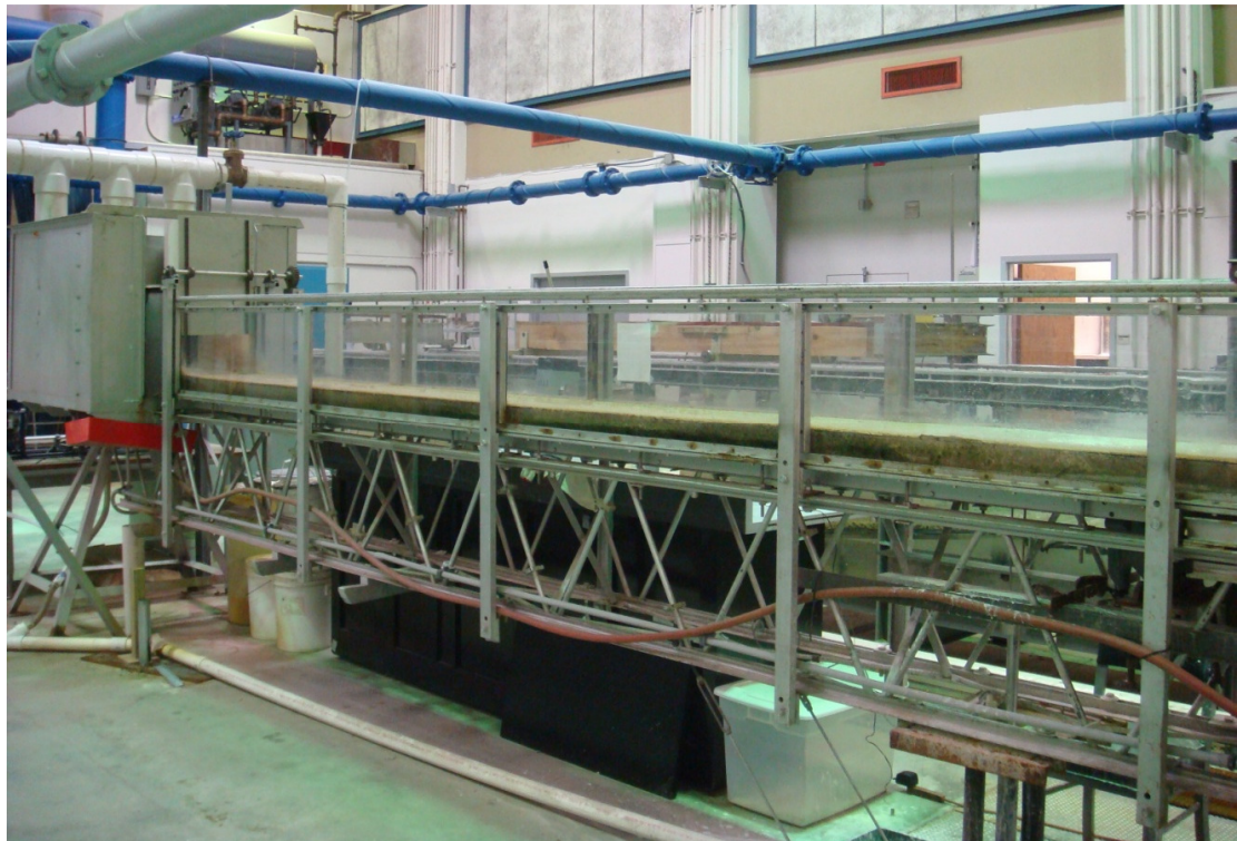
Figure 3.7 Flume apparatus for the erosion test: system layout (upper) and photo (lower)
