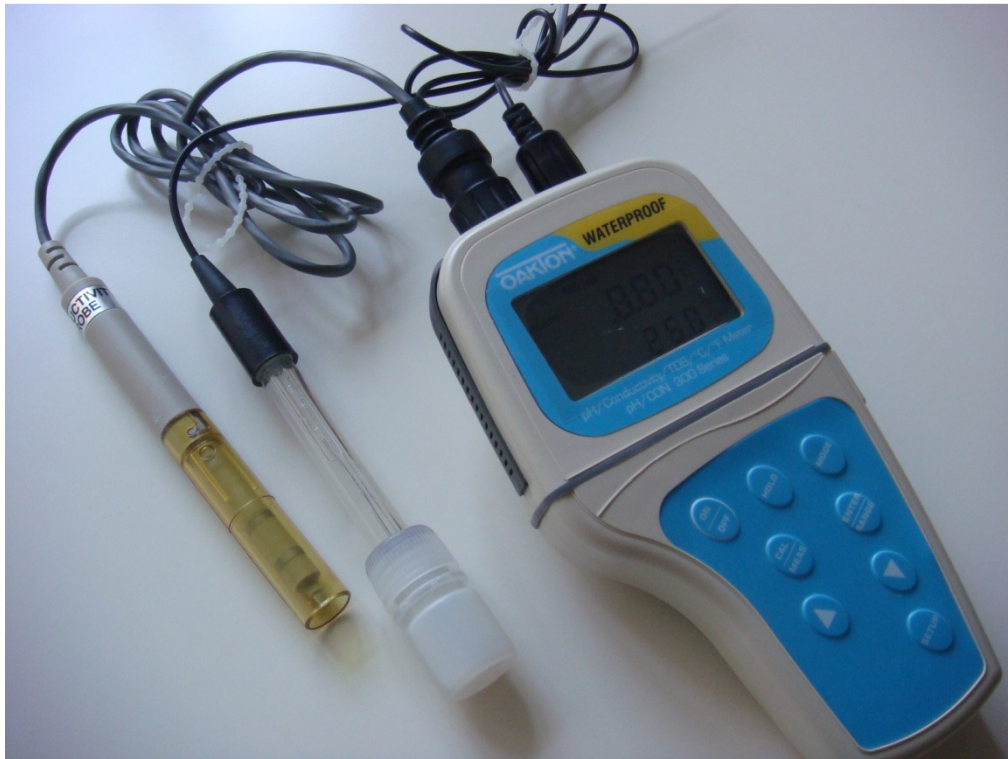
Figure 3.6 Oakton waterproof PC 300 hand-held pH/Conductivity/TDS/Temperature Meter
