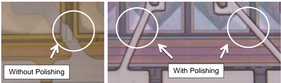
Figure 39. Similar electronics without polishing (left) and with polishing (right). The discontinuity of the connection line has been mitigated through the addition of silicon oxide and subsequent polishing.
