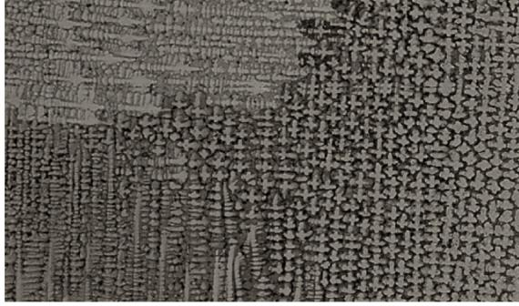
**Figure 72:** Image demonstrating the CET in which the columnar structure in the lower left transitions into the equiaxed structure on the right.
