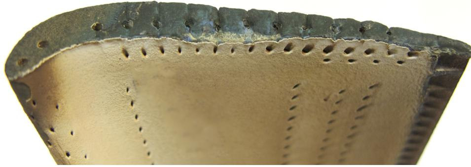
(a) Turbine engine airfoil illustrating wear at the blade tip.
