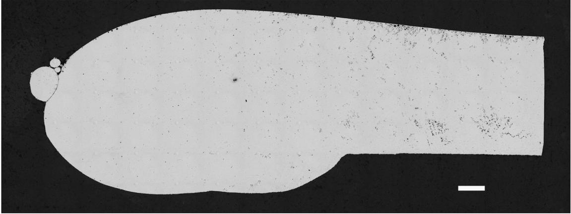
**Figure 94:** Micrograph of sample RENE15 demonstrating extreme substrate melting at high energy density with a high number of repeat scans. Scale bar is 1mm.
