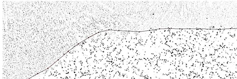
**Figure 52:** Closeup view of the René-80 meltback line [62].
