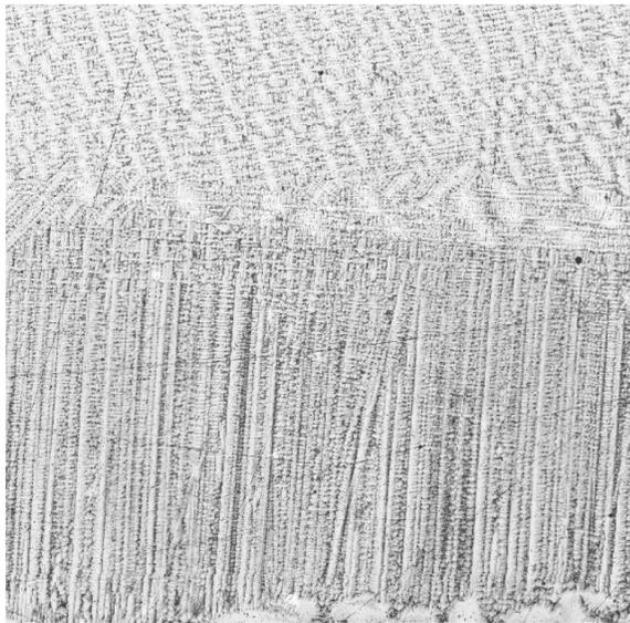
**Figure 73:** Image demonstrating the OMT indicated by the vertical columnar structure at the bottom of the image flipping to a horizontal columnar structure near the top of the image.
