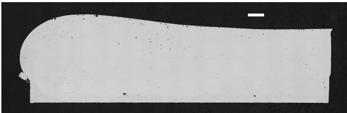
**Figure 92:** Micrograph of sample RENE14 demonstrating a highly uniform deposit height with sufficient but not excess melt back. Scale bar is 1mm.
