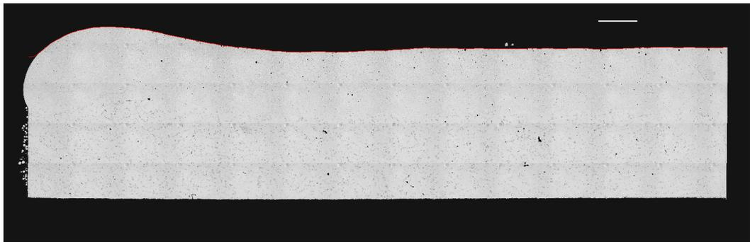
**Figure 125:** Micrograph of a sample run with a constant reference temperature of  $1650\text{ }^{\circ}\text{C}$  demonstrating a higher deposit height than the lower reference temperature. Scale bar of 1mm length.
