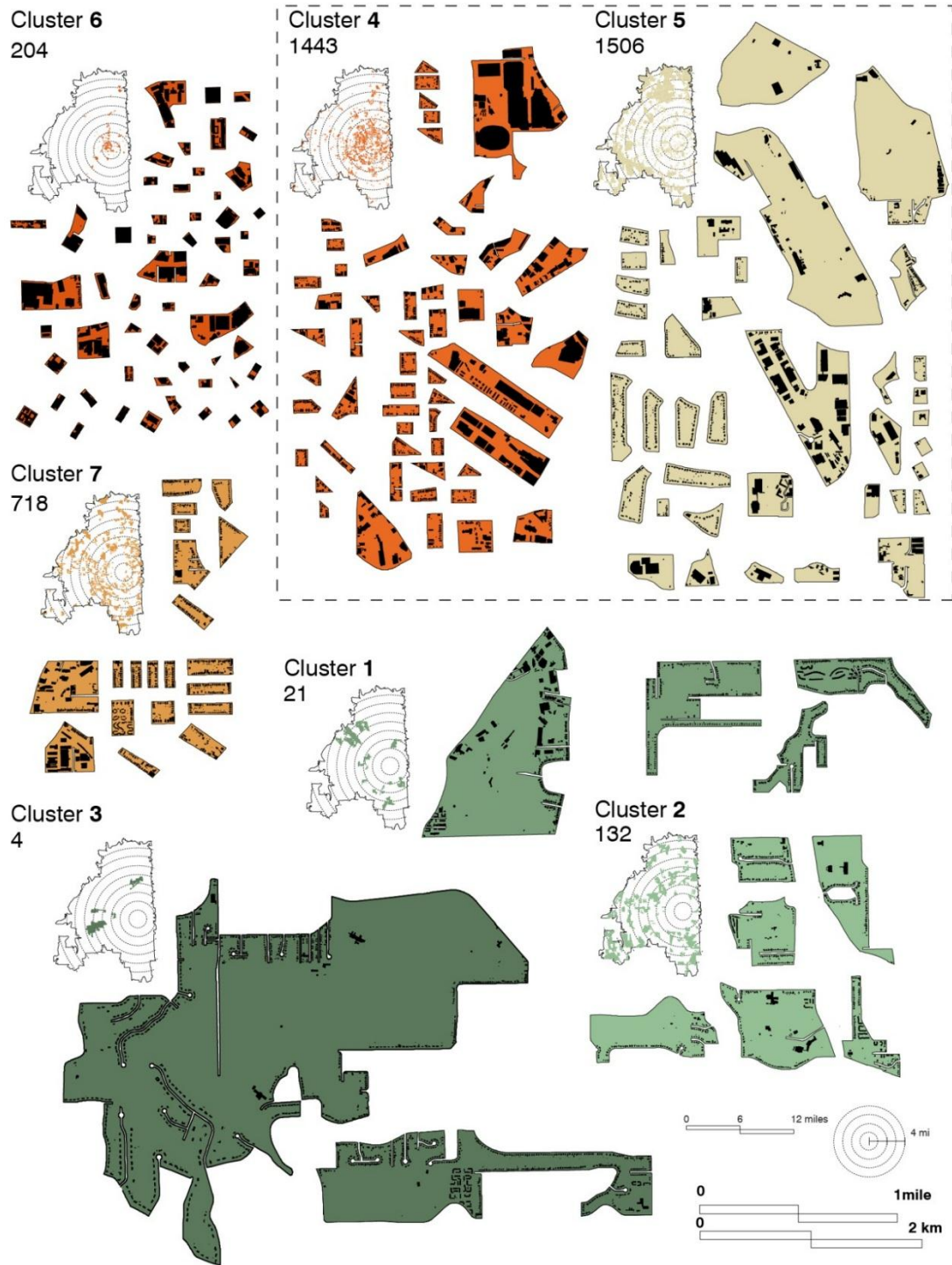
Figure 66. Clusters based on internal load which depict building configurations: their density, their location at the center or on the edges of the block (with the number of blocks in each cluster). The dotted line highlights blocks more likely to evolve.
