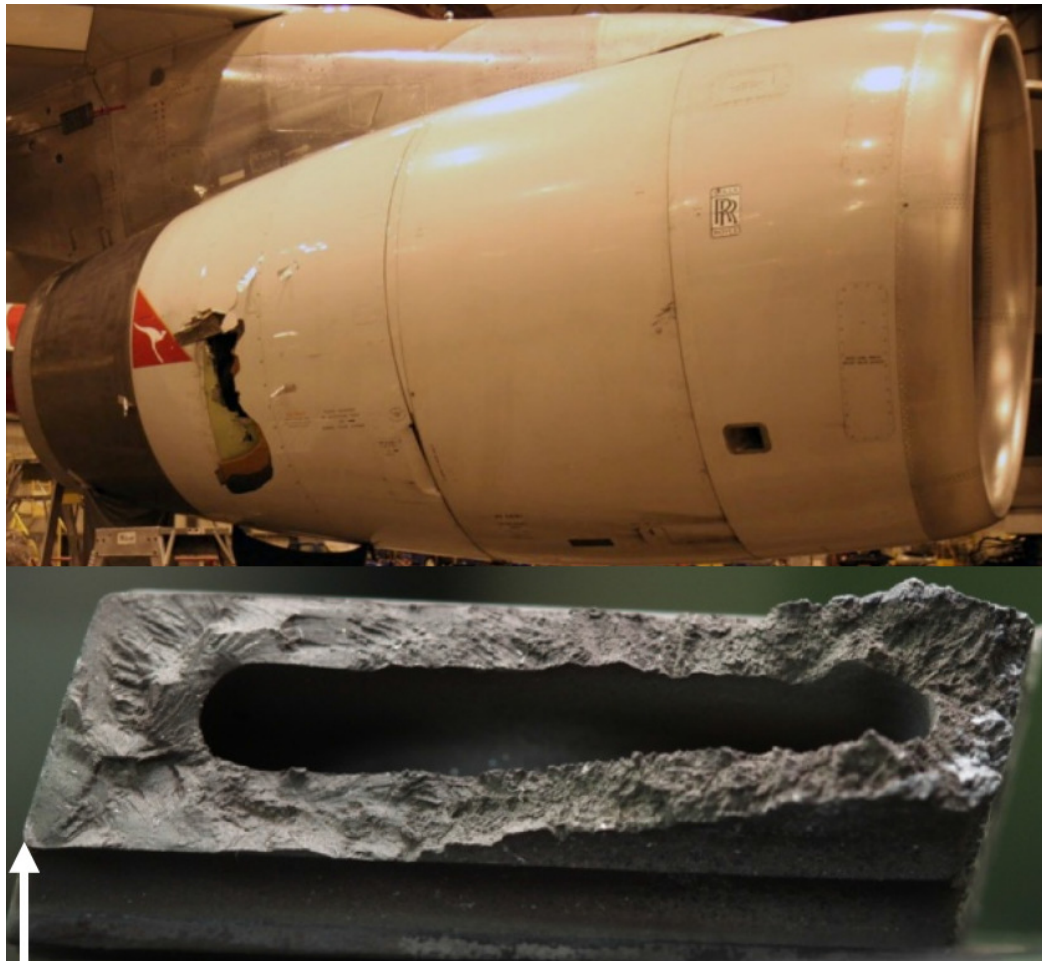
Figure 1.4: Turbopfan Engine Blade Failure: (Bottom) Fractured Blade Root (Top) Perforated Engine Nacelle [7]
