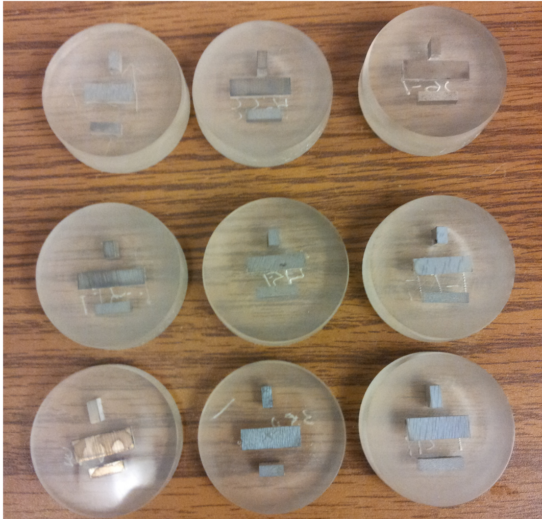
Figure 3.23: Mounted Specimens after Grinding, Polishing and Etching
