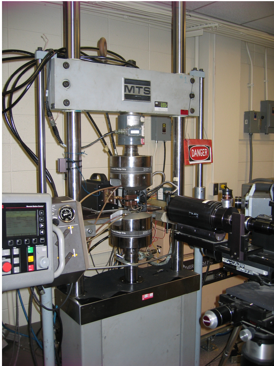
Figure 3.13: MTS Load Frame Used for Thermo-Mechanical Fatigue Testing
