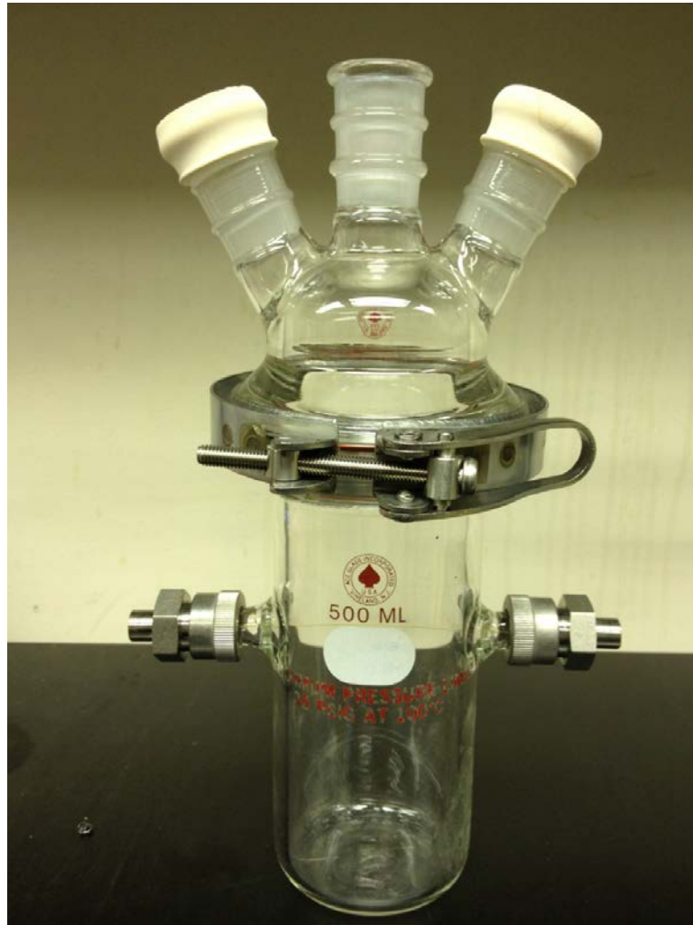
Figure 3-3. Illustration of pervaporation module.
