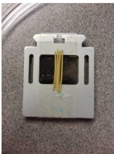
Figure 3-1. Illustration of mounted XRD sample.
