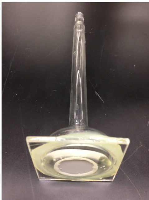
Figure 2-4. Illustration of disk membrane module for pervaporation experiments.
