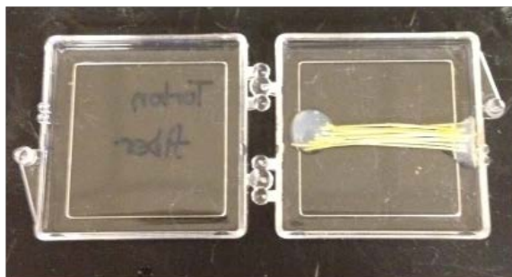
Figure 3-21. Illustration of mounted FT-ATR/IR sample.
