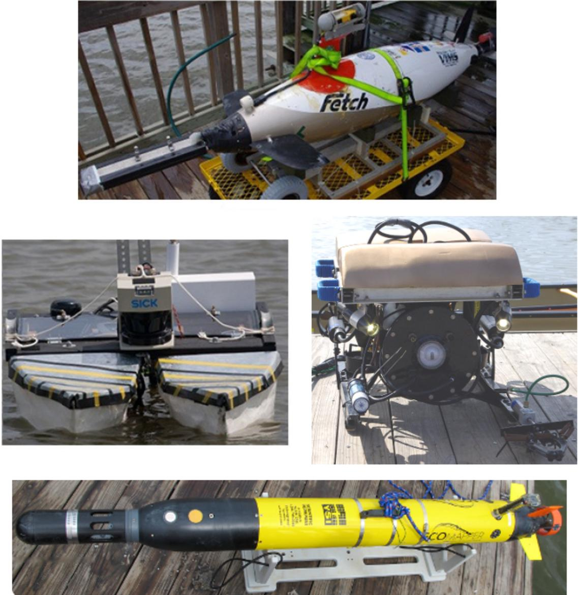
**Figure 28:** Marine vehicles used in the survey. From top to bottom: AUV-Fetch 1, ASV-Victoria (left), ROV- $\beta$  (right), and the EcoMapper.
