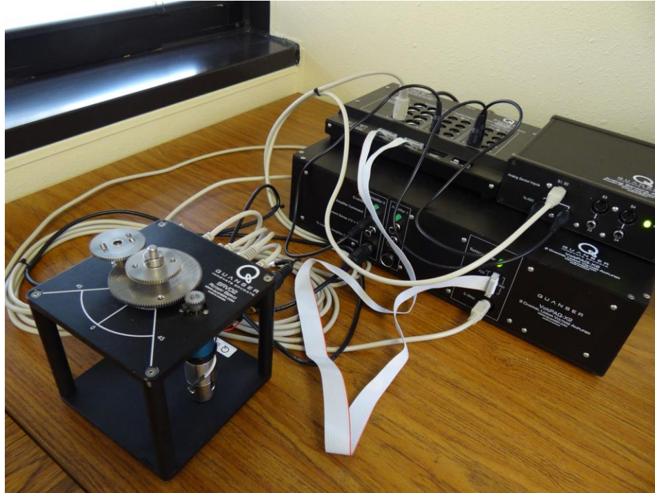
Fig. 35. Hardware connections between SRV-02, amplifier, and data acquisition board.
