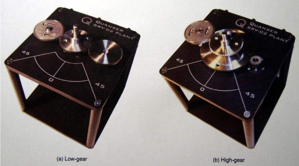
Fig. 34. Low and high-gear configurations of Quanser SRV-02 DC motor system.
