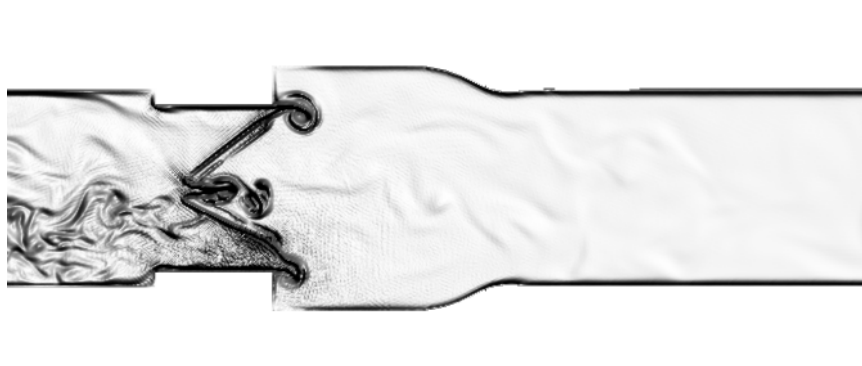
Figure 5-57: 2D vorticity plot showing leaflet opening from two-way FSI modeling
