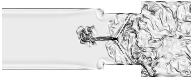
(a) Initial jet flowing centrally upon leaflet closure
