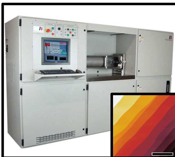
Figure 2.3: Commercial First Nano Graphene Furnace (Easy Tube 3000), capable of heating up to 100 mm diameter substrates up to 2200 °C in various environments. The inset is an AFM image of a 4H SiC(0001) substrate hydrogen etched in this furnace, displaying smooth and straight 8.43 \pm 2.68 nm high step bunches (scale bar is 20 \mu m)
