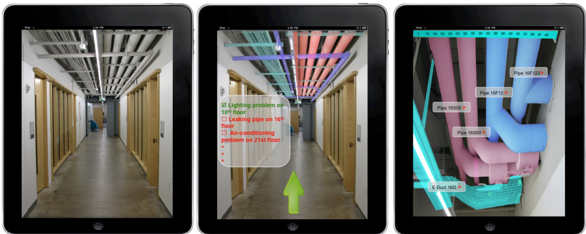
(a) Real-world view of the facility (b) Navigation and task list (c) Filtering information from BIM model
