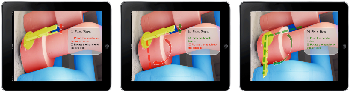
(a) Part 1: Pressing the handle (b) Part 2: Rotating the handle (c) Successful performance of part 1 and 2
