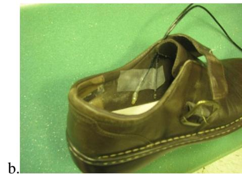
Figure 3.2 Temperature and RH sensor placement a. foot, b. shoe
