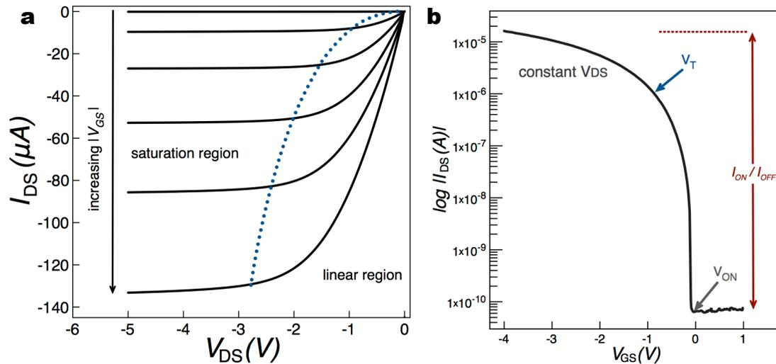
Figure 3.7. Typical curves of a p-type TFT. **a**, Output characteristics. **b**, Transfer characteristics.
