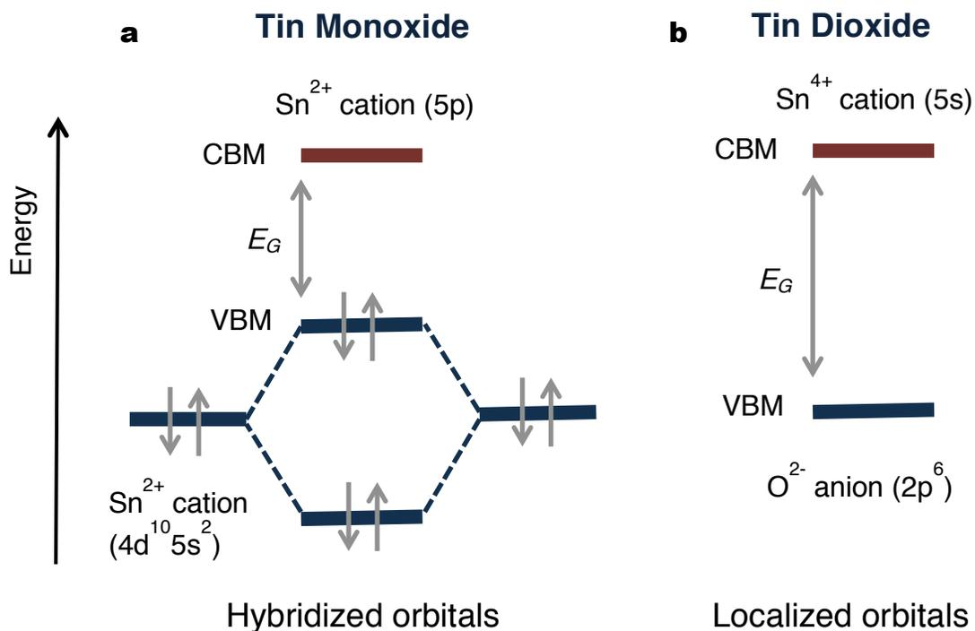
**Figure 2.10. Band structure comparison.** a, SnO b, SnO<sub>2</sub>. SnO shows orbital hybridization at the VBM while SnO<sub>2</sub> shows localized O 2p orbitals, characteristics of conventional n-type oxides.
