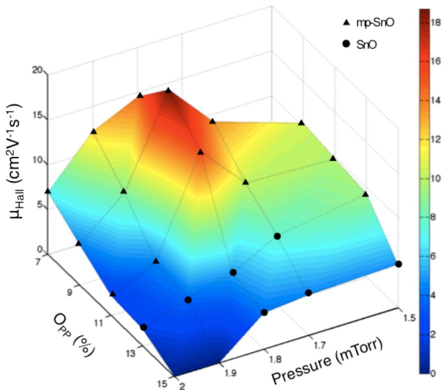
**Figure 4.4. Hall Mobility.** Room temperature Hall mobility of the films deposited in the pressure range from 1.5 mTorr to 2.0 mTorr and 7%  $O_{PP}$  to 15%  $O_{PP}$ . The point at 7%  $O_{PP}$ , 1.5 mTorr showing n-type conduction as well as the 15%  $O_{PP}$  at 1.9 mTorr and 2.0 mTorr showing unreliable measurements, are set to zero. A maximum Hall mobility of  $18.7 \text{ cm}^2\text{V}^{-1}\text{s}^{-1}$  is obtained at 1.8 mTorr, 9%  $O_{PP}$ .
