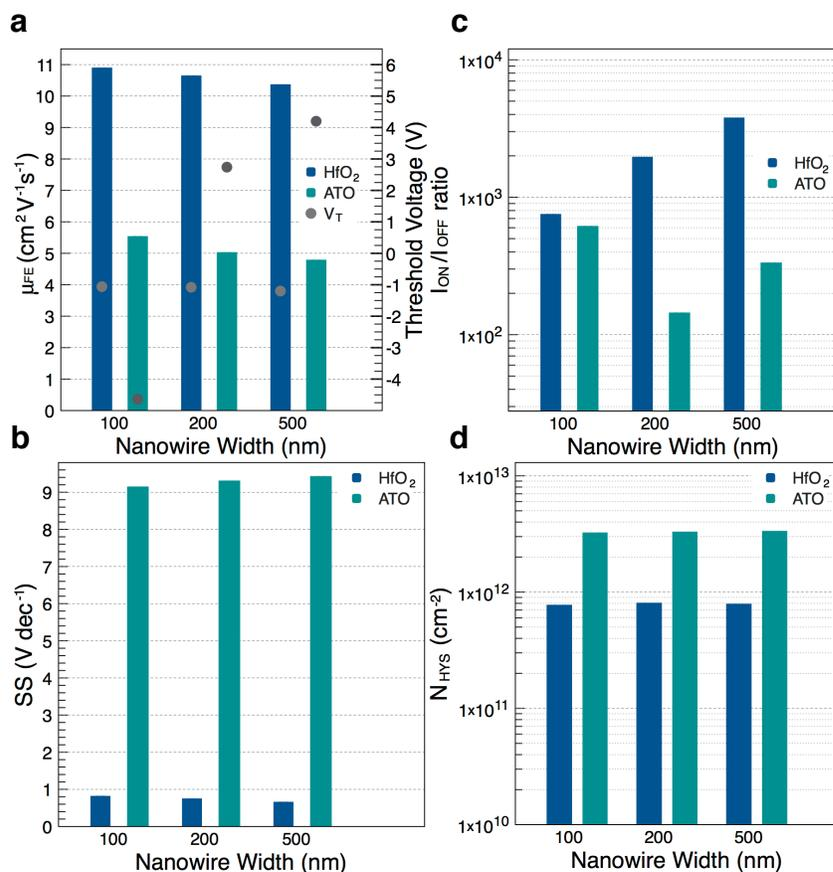
**Figure 5.7.** Effect of gate dielectric material on the performance of NW-FETs fabricated at the optimum anneal temperature (160 °C). **a**, field-effect mobility ( $\mu_{FE}$ ) and threshold voltage ( $V_T$ ); **b**, subthreshold swing (SS); **c**, on-to-off current ratio ( $I_{ON}/I_{OFF}$ ); **d**, effective hysteresis density ( $N_{HYS}$ ).
