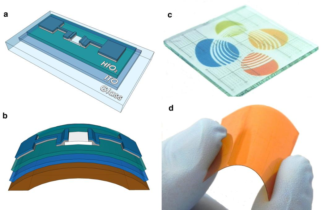
**Figure 4.7. Device structure.** Conceptual designs of the fabricated devices. **a**, fully transparent devices on glass and **b**, flexible devices on translucent polyimide (150 nm ITO gate electrode/220 nm HfO<sub>2</sub> gate dielectric/15 nm SnO<sub>x</sub> active channel/8 nm Ti, 90 nm ITO source and drain electrodes). Photograph of **c**, a fully transparent device and **d**, a flexible one.
