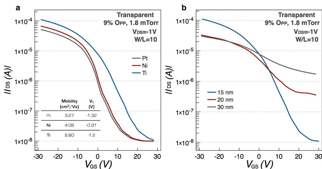
**Figure 4.11. Transfer characteristics for different conditions.** **a**, Different source and drain contacts **b**, Different thicknesses of the SnO active layer. All devices using HfO<sub>2</sub> as the gate dielectric and deposited on glass substrates.
