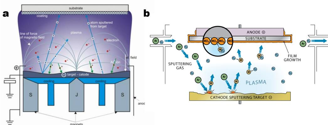
**Figure 3.1. Magnetron Sputtering.** **a**, Phenomena occurring during the sputtering process. *From Arzuffi SRL*<sup>5</sup>; **b**, Schematic of reactive sputtering. *From clear metals Inc.*<sup>6</sup>
