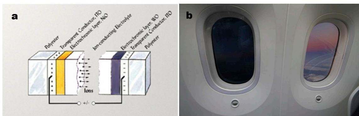
**Figure 2.6. Electrochromic device.** **a**, Basic device structure. *From Granqvist et al<sup>41</sup>*; **b**, Electronically adjustable windows in the Boeing 787 Dreamliner. *From theplaneblog.wordpress.com*.
