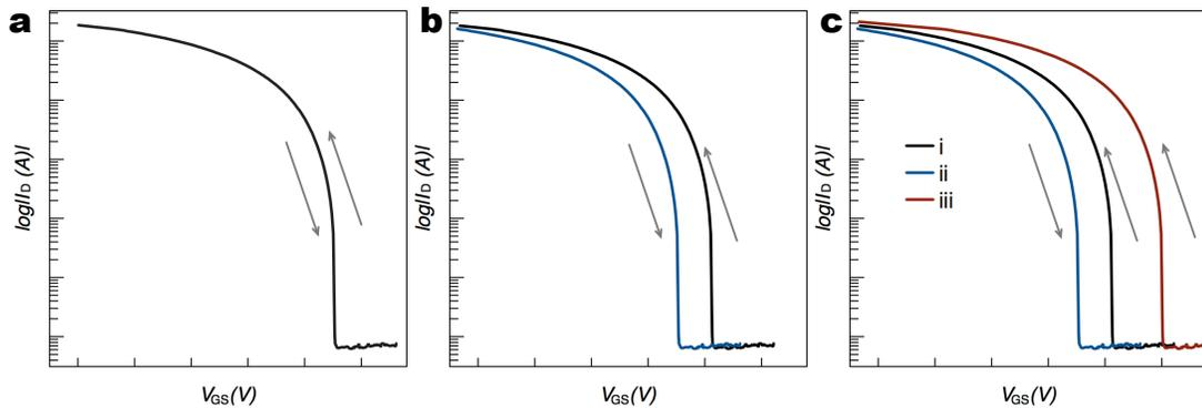
**Figure 3.10. TFT behavior.** Multiple dual-sweep transfer curves for **a**, equilibrium; **b**, non-equilibrium, steady-state; **c**, non-equilibrium, non-steady-state TFT operation. Adapted from Wager<sup>34</sup>.
