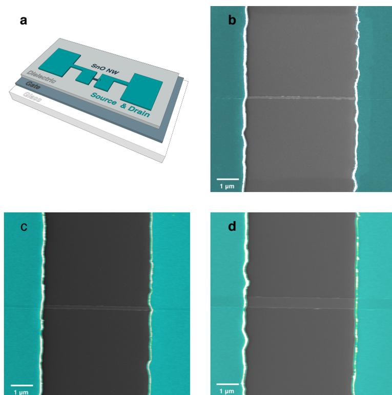
**Figure 5.1. Conceptual design and SEM images.** **a**, Conceptual design of the fabricated devices (150 nm ITO gate electrode/220 nm HfO<sub>2</sub>/ATO gate dielectric/ EBL-patterned SnO nanowire channel/8 nm Ti, 80 nm Au source and drain electrodes); Top view scanning electron microscopy image of fabricated device with channel length of 5  $\mu\text{m}$  and channel width defined by the nanowire planar width of **b**, 100 nm; **c**, 200 nm; and **d**, 500 nm.
