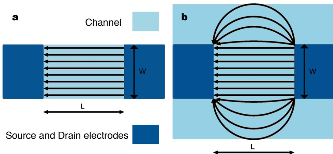
Figure 3.9. Current pathways in TFTs with identical drawn width ( $W$ ) and length ( $L$ ). a, Patterned channel. b, Unpatterned channel. Adapted from Hong *et al.*<sup>33</sup>
