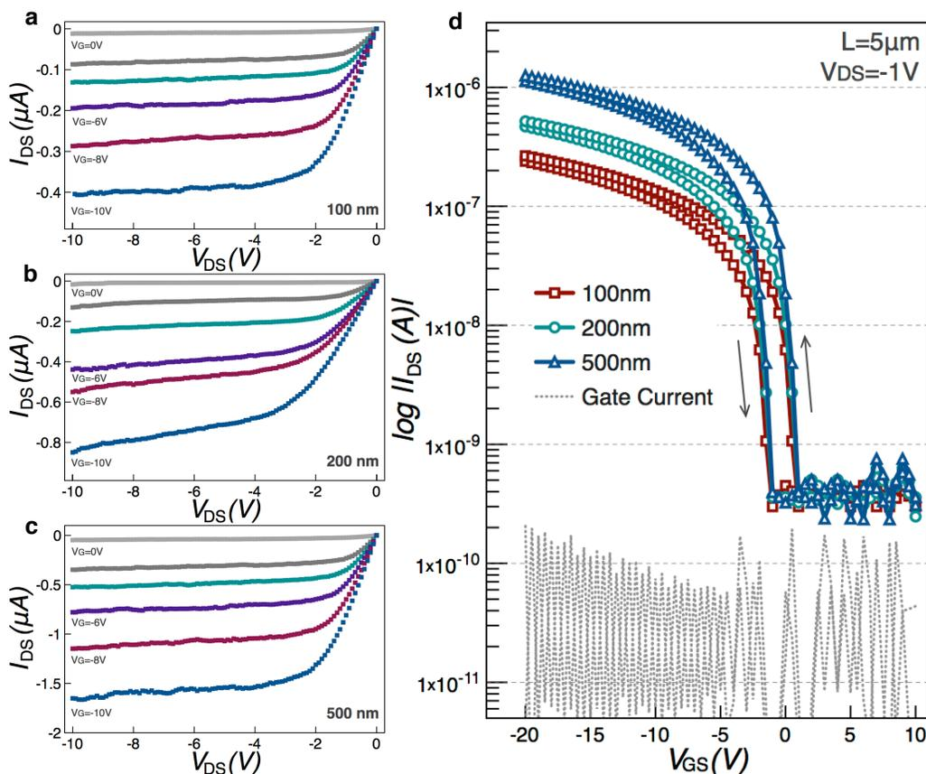
**Figure 5.3.** Output and transfer characteristics of devices annealed at  $160^\circ C$ . Output characteristics of devices **a**,  $100$  nm; **b**,  $200$  nm; and **c**,  $500$  nm nanowire transistors (NW-FETs) respectively; **d**, Transfer characteristics of NW-FETs as a function of nanowire width when using  $HfO_2$  as the gate dielectric.
