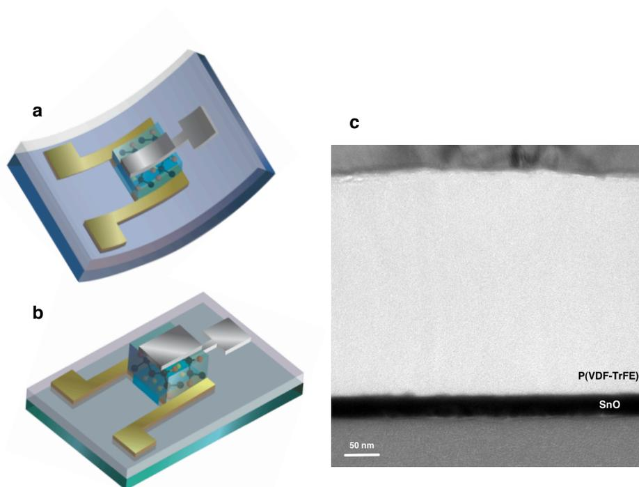
**Figure 6.1. Conceptual design of the devices.** **a**, polyimide substrate; **b**, glass substrate; **c**, TEM image of the SnO/P(VDF-TrFE) interface.
