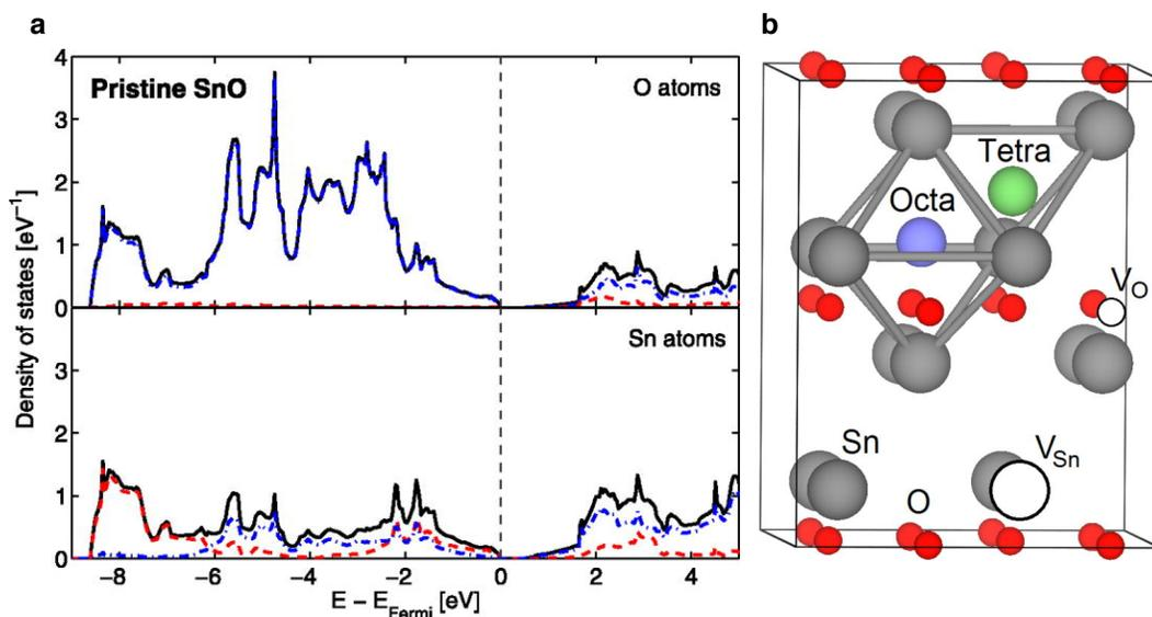
**Figure 4.5. Partial density of states of SnO and native defects. a,** Pure phase SnO. Black solid line: summed valence states (O  $2s+2p$  and Sn  $5s+5p+4d$ ), red dashed line: summed  $s$  states (O  $2s$  and Sn  $5s$ ), blue dashed-dotted line: summed  $p$  states (O  $2p$  and Sn  $5p$ ). Fermi energy is set to the top of the valence band. **b,** Native defects in SnO. From Granato *et al.*<sup>33</sup>
