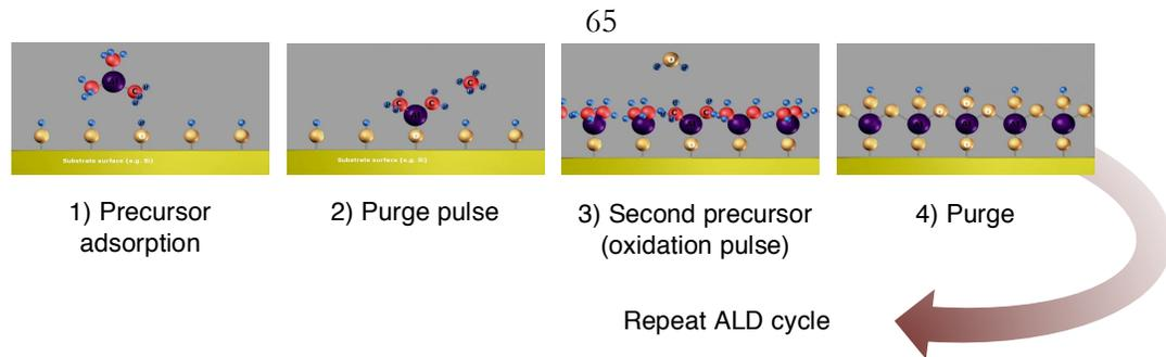
**Figure 3.3. ALD.** Four major steps in each cycle. *Adapted from [www.laserwort.com](http://www.laserwort.com)*
