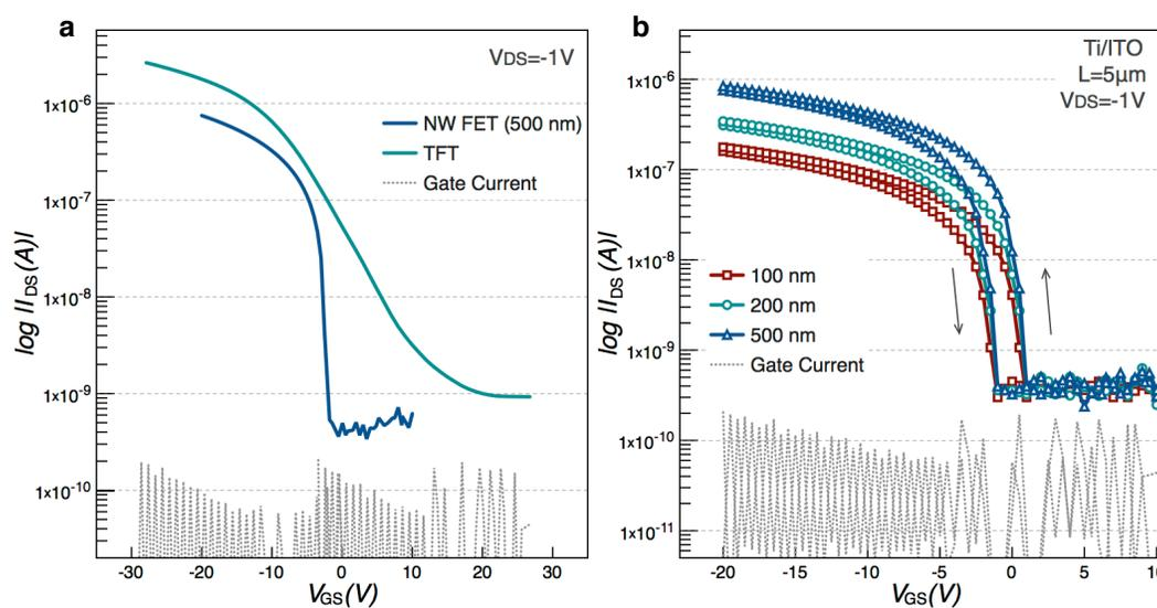
**Figure 5.4. Transfer characteristics comparison.** **a**, Thin film transistor versus nanowire FET (500 nm); **b**, Transfer characteristics of NW-FETs as a function of nanowire width when using  $\text{HfO}_2$  as the gate dielectric, annealed at  $160 \text{ }^\circ\text{C}$  using Ti/ITO source and drain contacts.
