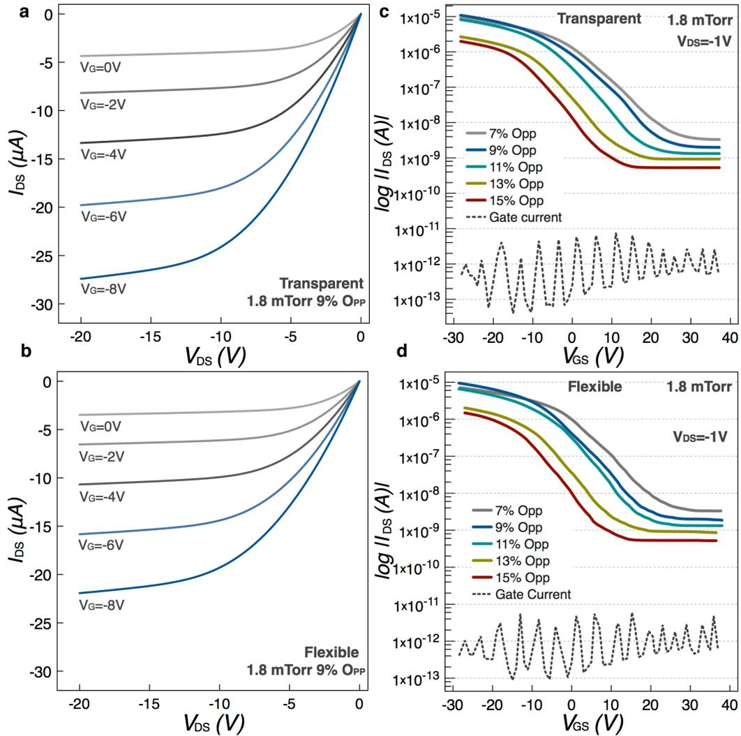
**Figure 4.8. Transfer and output characteristics.** a,b, Output and transfer characteristics of devices fabricated on glass (fully transparent) and c,d, devices fabricated on polyimide (flexible) with a channel width of  $50\ \mu\text{m}$  and length of  $50\ \mu\text{m}$ .
