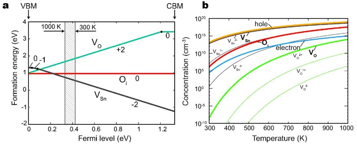
**Figure 2.11. Defect formation energy.** **a**, Defect formation energies as a function of the Fermi level. **b**, Defect concentrations as function of temperature. *From Togo et al.<sup>57</sup>.*
