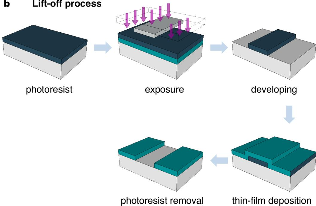
Figure 3.6. Photolithography processes. **a**, Conventional process flow. **b**, Lift-off process
