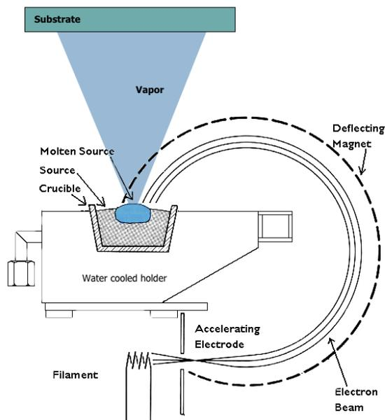
**Figure 3.2. E-beam evaporation.** Thin-film deposition by e-beam evaporation. *Adapted from* <http://www.cleanroom.byu.edu/metal.phtml>
