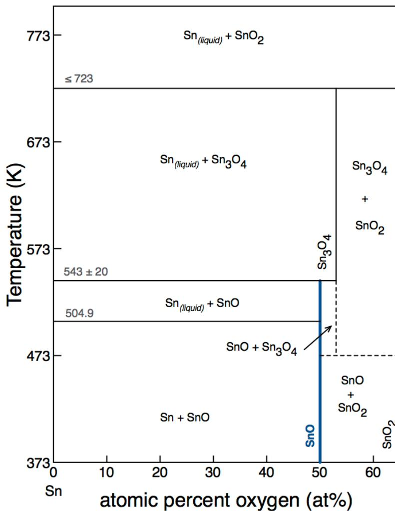
**Figure 2.7. Sn-O phase diagram.** Tin monoxide is observed as stoichiometric compound with a single, well-defined composition (highlighted in blue).
