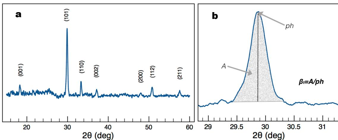
**Figure 3.4. XRD Pattern.** **a**, XRD pattern of single phase SnO, showing seven diffraction conditions. **b**, The integral breadth ( $\beta$ ) defined as the total area under the peak ( $A$ ) divided by the peak height ( $ph$ ), was obtained for every observed diffraction condition.
