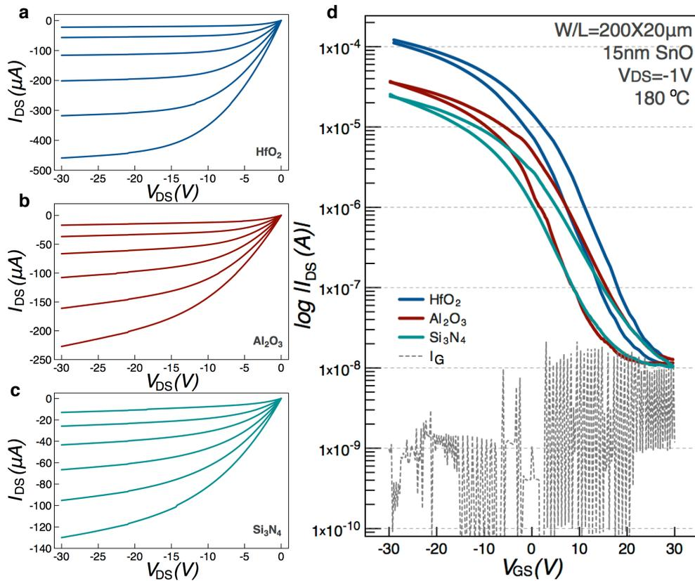
**Figure 4.12. Output and transfer characteristics for different gate dielectrics.** Output characteristics ( $V_G$  from 0 to -15 V at -3 V steps) for **a**, HfO<sub>2</sub>; **b**, Al<sub>2</sub>O<sub>3</sub>; **c**, Si<sub>3</sub>N<sub>4</sub>; **d**, Transfer characteristics as a function of gate dielectric. All devices using ITO as gate electrode, 15 nm thick SnO, Ti/ITO source and drain electrodes and deposited on glass substrates.
