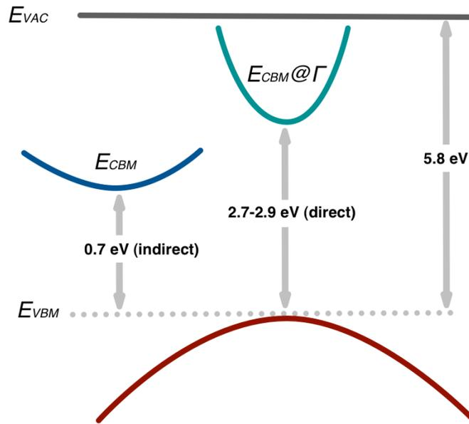
**Figure 2.12.** Schematic illustration of the band structure of SnO. Adapted from Nomura *et al.*<sup>1</sup>.
