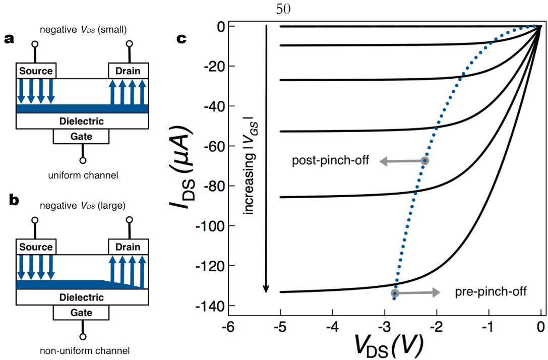
**Figure 2.16 Channel in the ON-state.** Schematics of TFT operation regions in the ON-state. **a**, Linear region, pre-pinch-off ( $-V_{DS} \leq -V_{GS} + V_T$ ); **b**, saturation region, post-pinch-off ( $-V_{DS} > -V_{GS} + V_T$ ). **c**, plot of  $I_{DS}$  versus  $V_{DS}$  for different  $V_{GS}$ .
