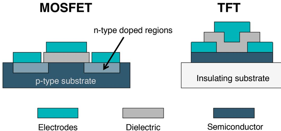
**Figure 2.14. Comparison between typical structures of TFTs and MOSFETs.** The single crystal Si wafer used in MOSFETs is both the substrate and the semiconductor.
