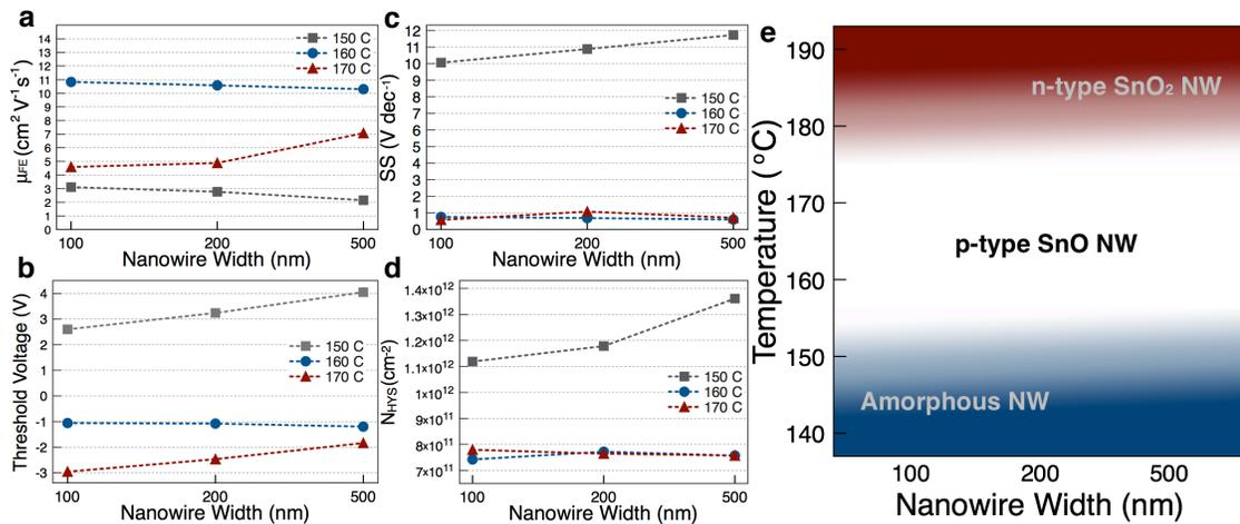
**Figure 5.6. Important NW-FET parameters measured as a function of nanowire width and anneal temperature. a,** field-effect mobility ( $\mu_{\text{FE}}$ ); **b,** threshold voltage ( $V_{\text{T}}$ ); **c,** subthreshold swing (SS); **c,** effective hysteresis density ( $N_{\text{HYS}}$ ). All devices shown here were fabricated using  $\text{HfO}_2$  gate dielectric. **e,** Process map depicting process conditions where p-type conduction is observed in SnO NW FETs.
