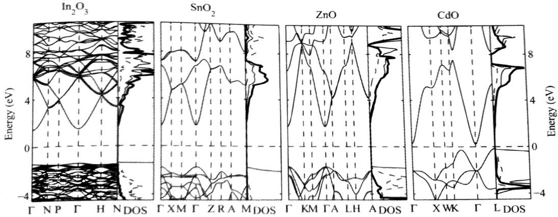
**Figure 2.1. Band structure of conventional TCO host materials.** Electronic band structure and partial density of states (DOS) of **a**,  $\text{In}_2\text{O}_3$ ; **b**,  $\text{SnO}_2$ ; **c**,  $\text{ZnO}$ ; **d**,  $\text{CdO}$ . In the DOS plots, the thick, dashed, and the thin lines represent metal  $s$ , metal  $p$  and oxygen  $p$  states, respectively. *From Facchetti and Marks<sup>2</sup>.*
