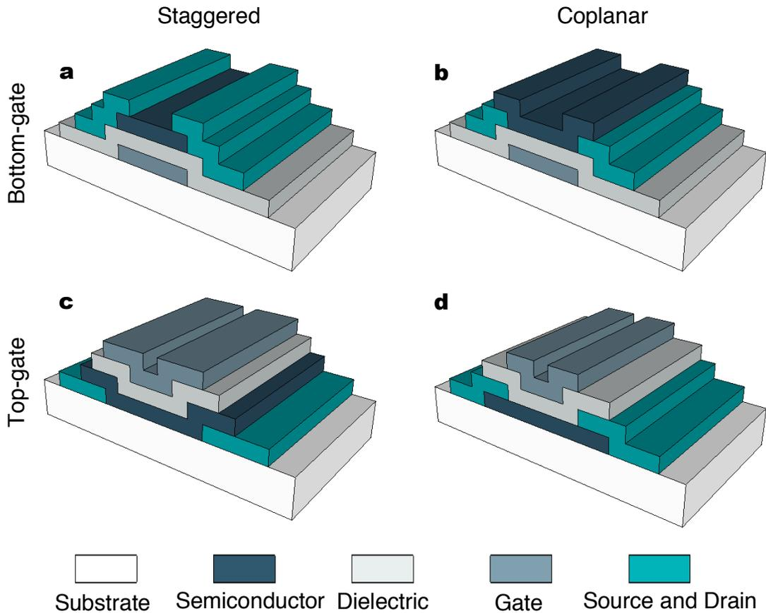
**Figure 2.13 Conventional TFT structures.** **a**, Staggered bottom-gate; **b**, coplanar bottom-gate; **c**, staggered top-gate. **d**, coplanar top-gate.
