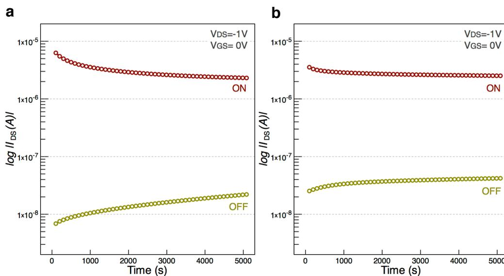
**Figure 6.4. Retention characteristics.** **a**, Rigid device; **b**, Flexible device. The ON/OFF states were produced at gate voltages of -30/+30 V with a 1 sec pulse and the retention was measured at zero gate bias condition.
