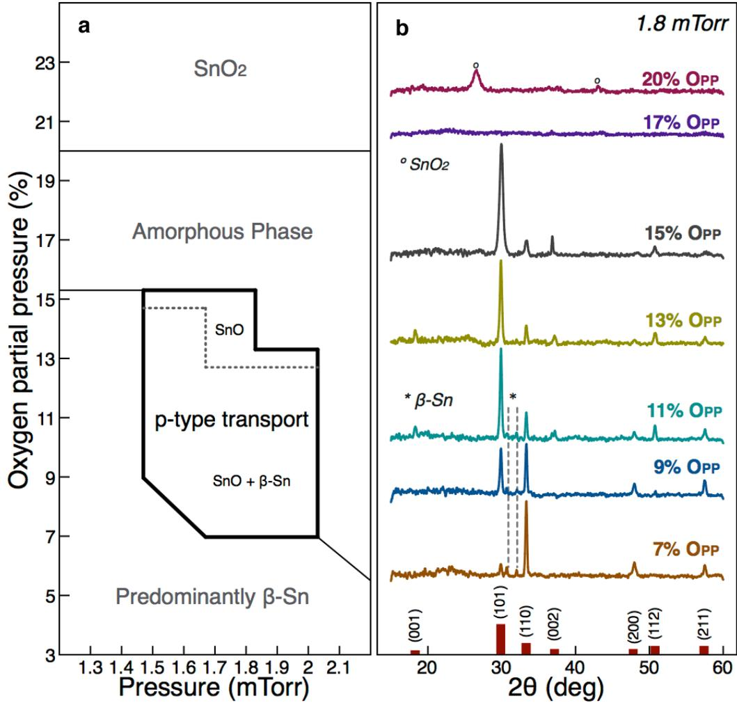
**Figure 4.1. SnO deposition map and XRD patterns.** **a**, phase stability map to obtain p-type tin oxide, which occurs in a very narrow window of deposition conditions. **b**, Phase formation dependence on the oxygen partial pressure ( $O_{pp}$ ) at a deposition pressure of 1.8 mTorr.
