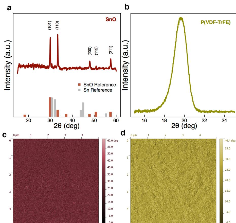
**Figure 6.3. Materials characterization.** **a**, XRD pattern of SnO thin films. The lines at the bottom show the diffraction patterns of tetragonal SnO (JCPDS card No. 06-0395) and tetragonal Sn (JCPDS card No. 04-0673); **b**, GIXRD pattern of P(VDF-TrFE) layer; **c**, AFM image of the SnO surface; **d**, AFM image of the P(VDF-TrFE) surface morphology.
