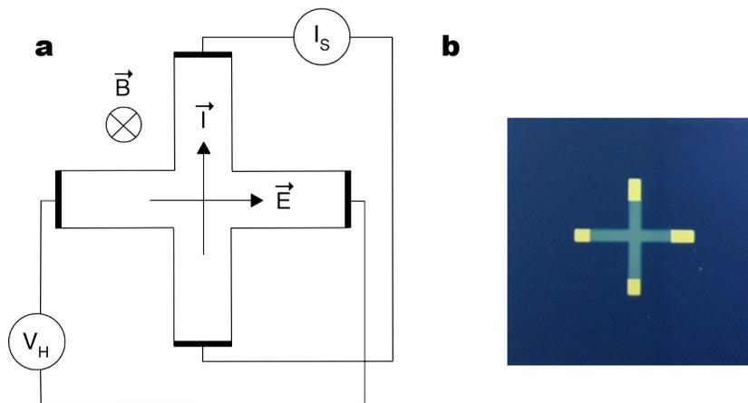
**Figure 3.5. Hall Effect.** **a**, Greek cross configuration used for measurements. **b**, Fabricated sample for Hall effect measurement.
