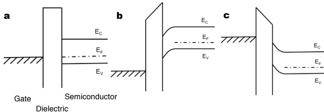
**Figure 2.15 Energy band diagrams.** A MOS capacitor with a p-type semiconductor under different gate bias: **a**, equilibrium ( $V_{GS}=0$  V); **b**, depletion ( $V_{GS}>0$  V); **c**, accumulation ( $V_{GS}<0$  V).
