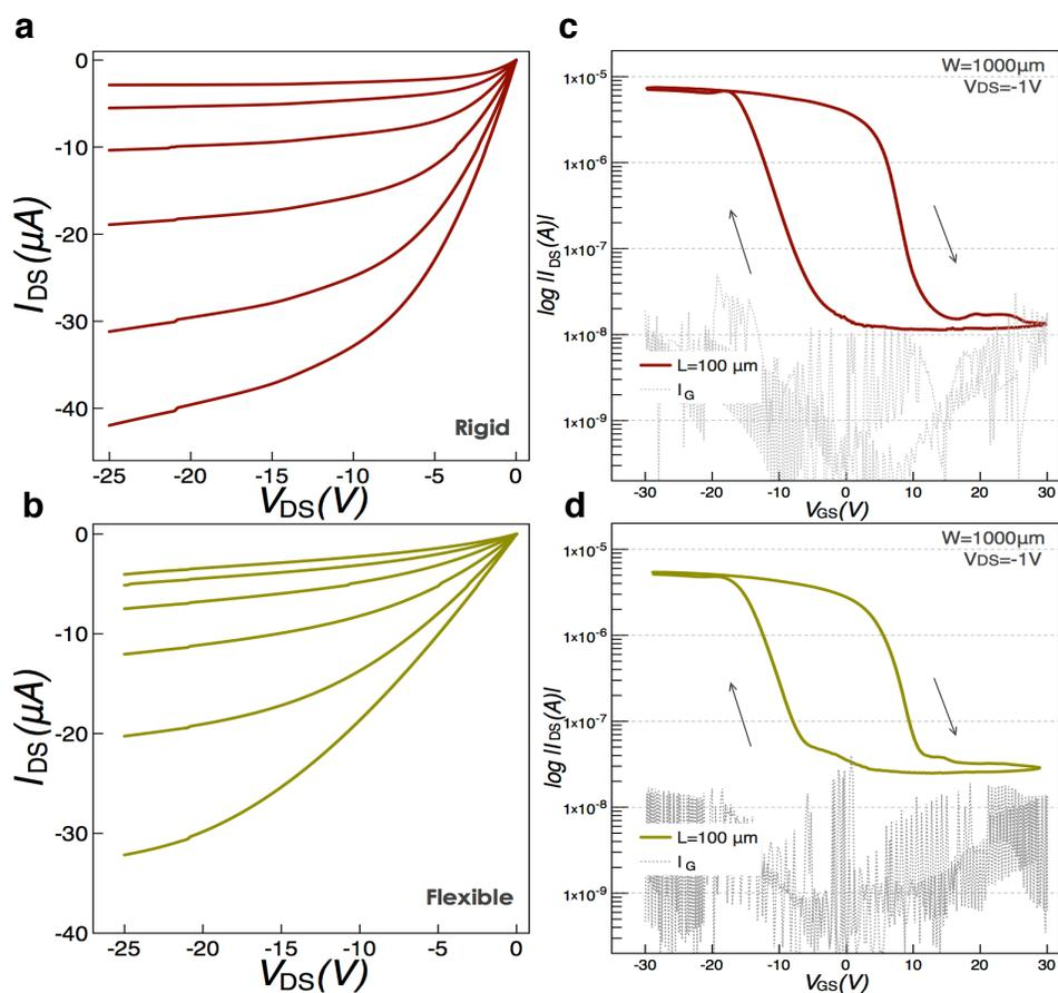
**Figure 6.2. FeFET static characteristics.** Output characteristics from  $V_{GS}=0 V$  to  $-15 V$  at  $-3V$  steps of **a**, glass substrate; **b**, polyimide substrate; Transfer characteristics at  $V_{DS}=-1V$  of **c**, rigid device; **d**, flexible device.
