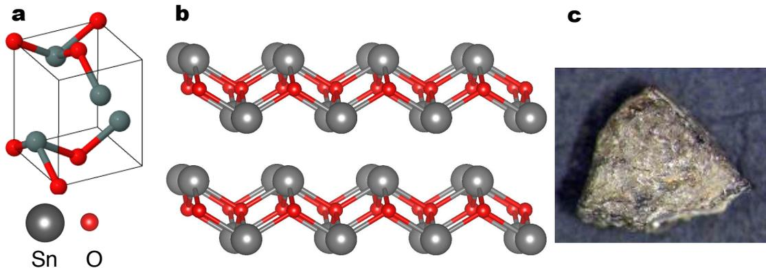
**Figure 2.8. Crystal structure of SnO.** **a**, Unit Cell; **b**, layered structure in the  $[001]$  crystallographic direction; **c**, Romarchite mineral, *from mindat.org*.
