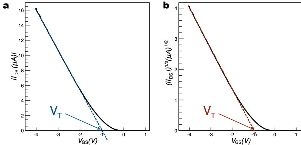
**Figure 3.8. Threshold Voltage ( $V_T$ ) extraction by linear extrapolation. a**, Linear region from  $I_{DS}$ - $V_{GS}$  curve. **b**, Saturation region from  $(I_{DS})^{1/2}$ - $V_{GS}$  curve.
