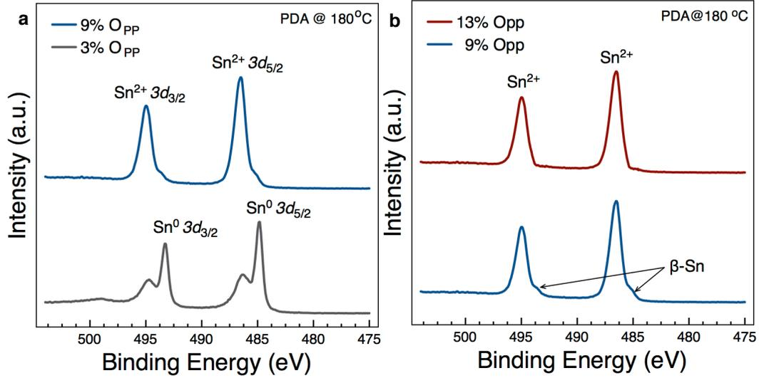
**Figure 4.3. XPS Analysis.** **a**, Films deposited at 3%  $O_{PP}$  and 9%  $O_{PP}$  and  $P=1.8$  mTorr after PDA at 180 °C. **b**, Post annealed films deposited at different  $O_{PP}$  showing the mixed phase condition (9%  $O_{PP}$ , 3 at% Sn) and single phase SnO (13%  $O_{PP}$ )
