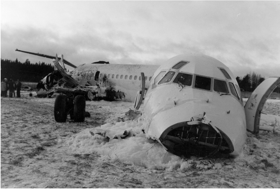
Figure 1.2: SAS SK751 wreckage at Gottröra, a crash caused by ice breaking off from the wings damaging the engines, or, is inappropriate human interaction with automated systems a more plausible explanation? (Photo: SHK)
