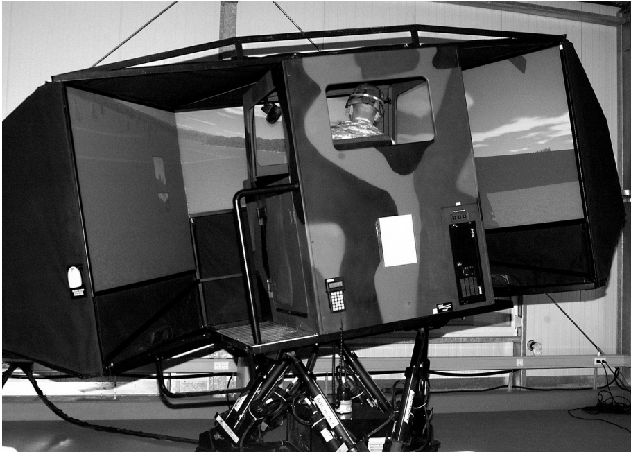
Figure 3.1: An example of a simulator for both visual and motion cues. (Source: wikimedia, public domain)
