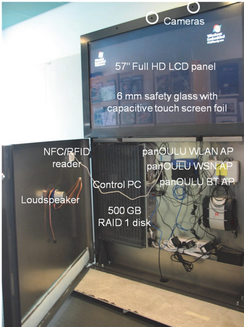
Figure 1. Components of an indoor hotspot.
