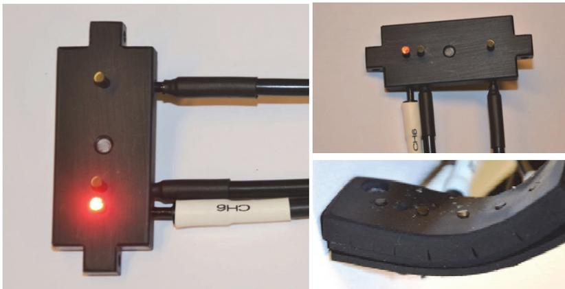
**Fig. 8. Fibre clips. On the left and upper right corner, a source fibre and two detector fibres attached at a distance of 5mm and 30 mm, respectively, from it. On the lower right corner is shown a clip version, made of flexible rubber, with five detectors. The thickness of the fibre output is 2.5 mm, and it is bent to a 90 degree angle.**
