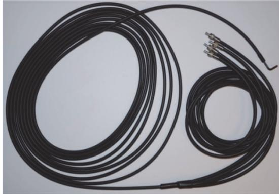
**Fig. 7. Fibre bundle with four inputs (male SMA connectors). Light from the four sources is guided to one fibre output with a 90 degree bend. The diameter of the fibre tip is 2.5mm.**
