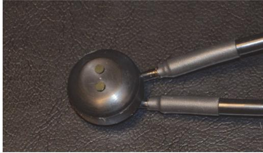
**Fig. 13. Optical probe or optode. Fibre tips of two MR-compatible fibres are on a fibre holder, made of olyOxyMethylene plastic, to provide a stable mounting for fibres at a distance of 5 mm from each other.**
