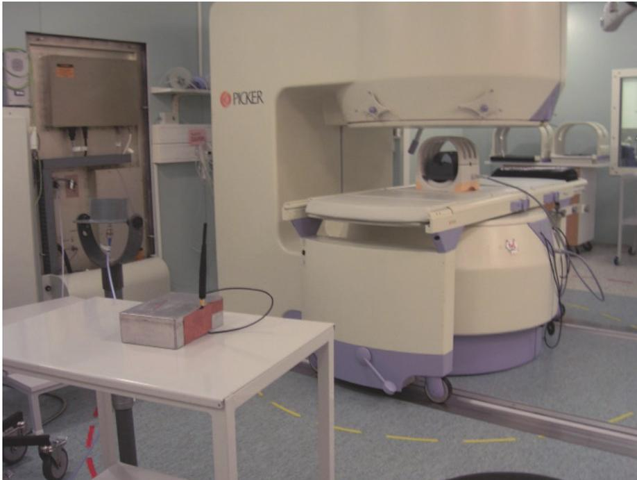
**Fig. 3. Test setup in the MRI room. Wireless SRDs are placed on the table near the MRI scanner (Paper I, published with the permission of © 2007 by University of Oulu).**
