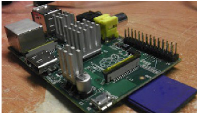
Fig 24. A set of dissipators and heat-sinks on an ARM-based SoC, the Raspberry Pi.
