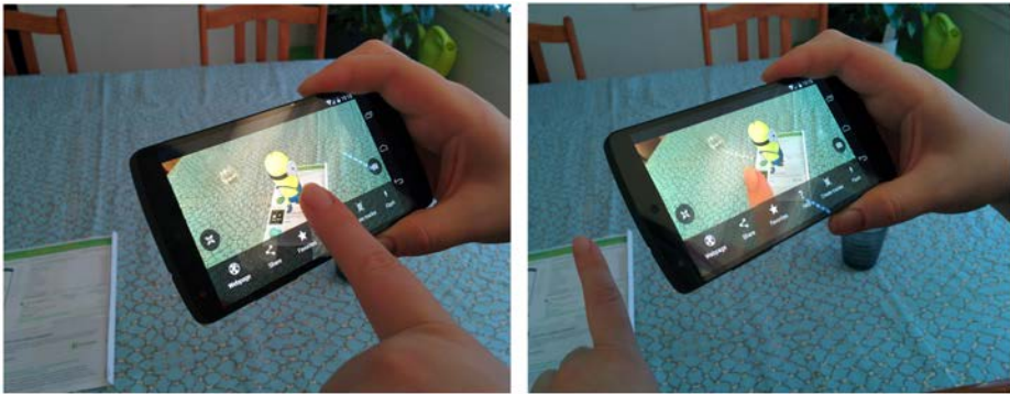
Fig 10. Potential problems with mobile interactivity via a touch screen. The hand or finger partially obstructs the view, and two handed operations are needed.
