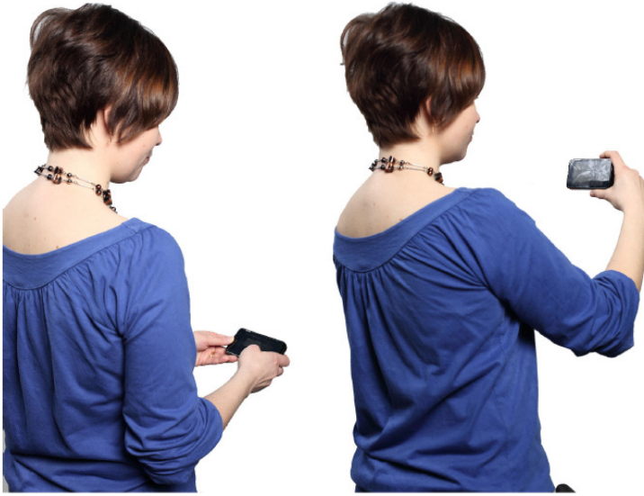
Fig 36. Automatic launching of a camera application. When the device is raised in front of the user and a face is in the field of view, the main camera starts the capture. (Bordallo López et al. 2012b) ©Springer.
