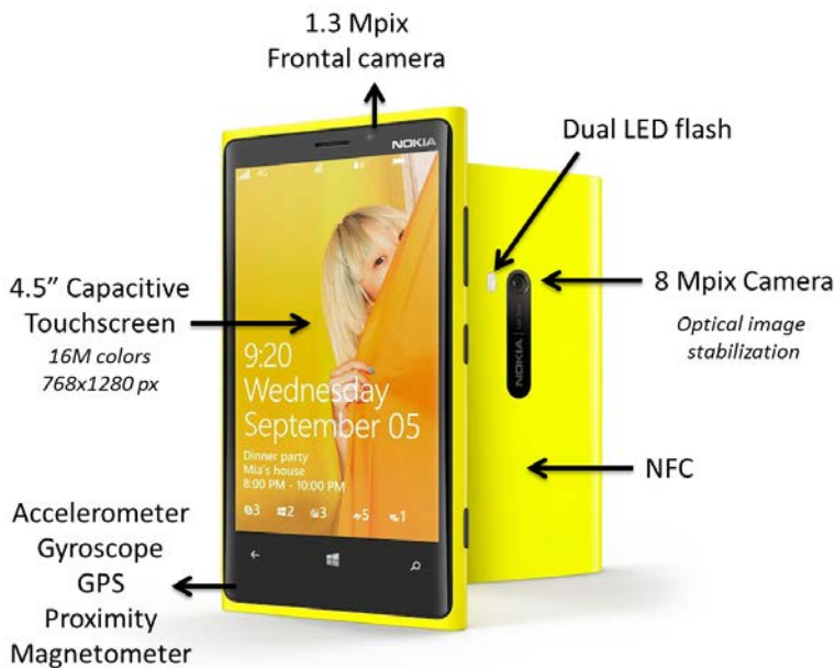
Fig 1. Nokia Lumia 920. Current mobile devices include several cameras, sensors, and a large display within a very constrained space.
