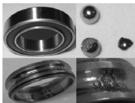
Fig. 7.2: Photos of degraded bearings from Nectoux et al. (2012)
