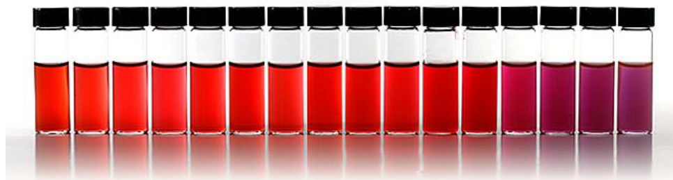
Figure 7. Aqueous suspensions of gold nanospheres from 5 to 100 nm in diameter (from nanoComposix ® ) [124].
