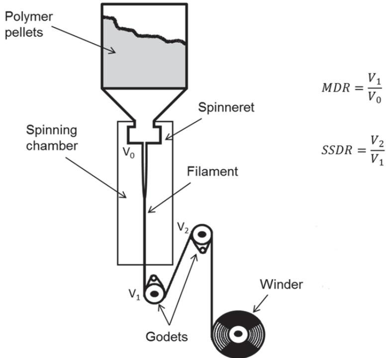
**Fig. 4. Schematic view of melt spinning process. The molten polymer is extruded into an air stream, which cools the melt and solidifies the filament under melt draw ratio (MDR), where  $V_0$  is the filament speed at the spinneret exit and  $V_1$  is the filament speed at the first godet. The filament is further undergoing solid-state drawing (SSD) under temperature controlled godets, where  $v_2$  is the speed at the second godet.**
