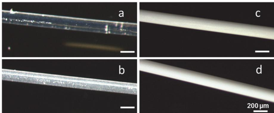
Fig. 5. Optical micrographs of PLA monofilament fibers showing that they become opaque with increasing SSDR, a) SSDR 3, b) SSDR 4, c) SSDR 5 and d) SSDR 6. Scale bar = 200 μm. (Paper I)
