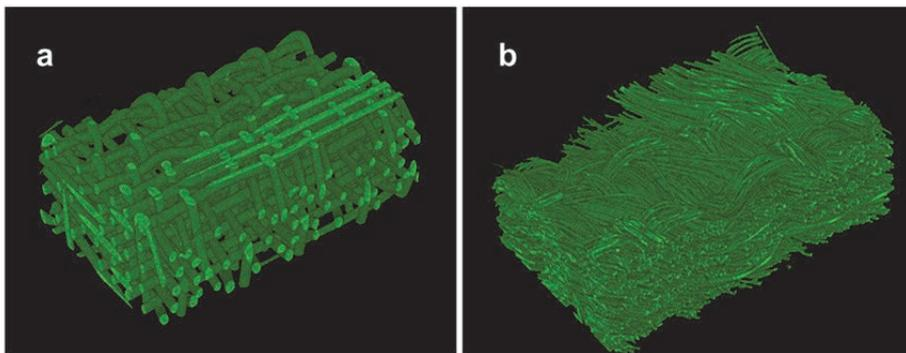
**Fig. 7. MicroCT reconstruction of PLA textile structures, a) monofilament fibers and, b) multifilament fibers in all three directions**
