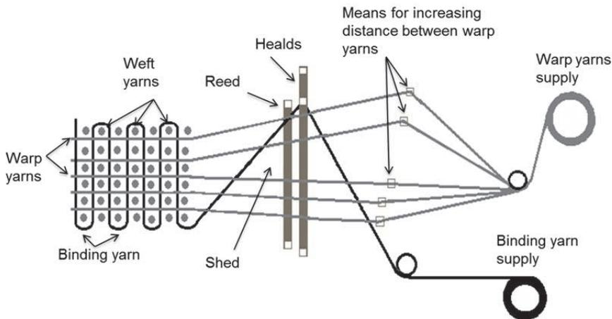
**Fig. 3. Schematic view of 3D weaving. Modified from Hu 2008b**
