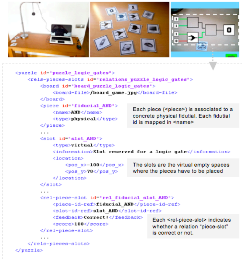
Figure 14. Example of using the XML binding for representing the tangible puzzle board game for computer architecture concepts
