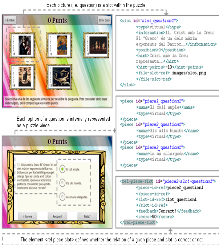
Figure 34. Sample of the XML representation compliant with the model used in “QuesTInSitu: The Game” (MNAC version)
