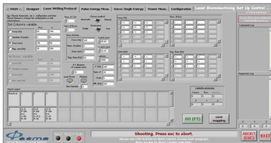
FIGURE A-7: The “Laser Writing Protocol” window for the evaluation of the material ablation procedure at different conditions (pulse energy, number of pulses, repetition rate and z position-focus).
