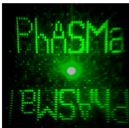
FIGURE 3-51: Reconstruction of the QD-doped polystyrene CGH using a 532 nm laser source. The distance between the CGH and the screen is about 10 cm.
