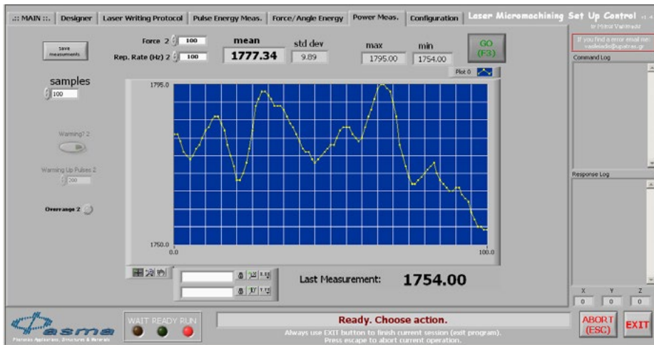
FIGURE A-10: The “Pulse Energy Meas.” window in time trace mode for monitoring the laser stability.
