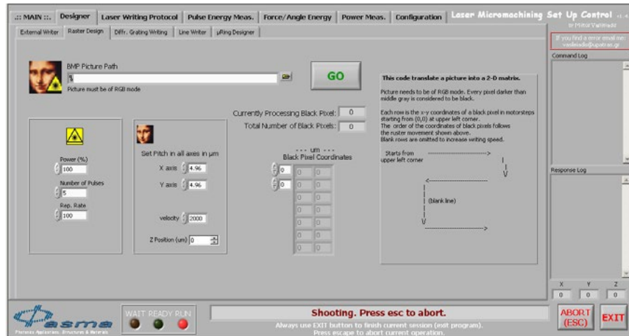
FIGURE A-3: The “Raster Design” window for inserting a jpg image file containing black and white pixels. The black pixels indicate the spots to be laser etched. The number pitch distances between pixels to be written and the force/number of pulses at each pixel are defined.
