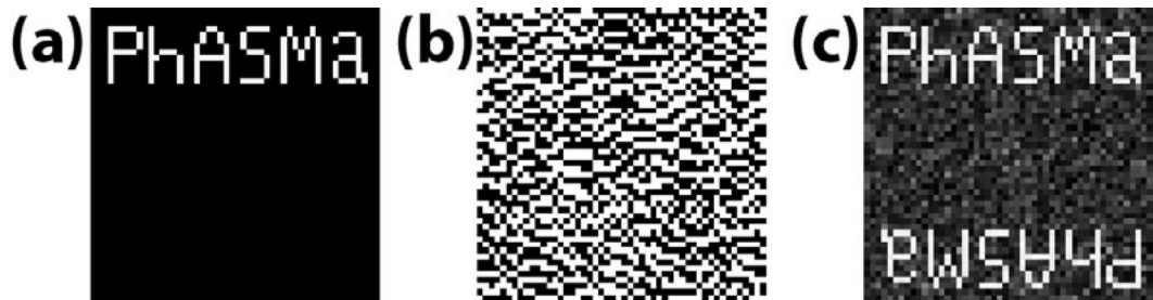
FIGURE 3-10: (a) Target design of a “PhASMA” logo CGH, (b) the optimum unit mask as calculated by the algorithm and, (c) the resultant reconstruction of the optimum mask of the CGH as predicted by the algorithm.
