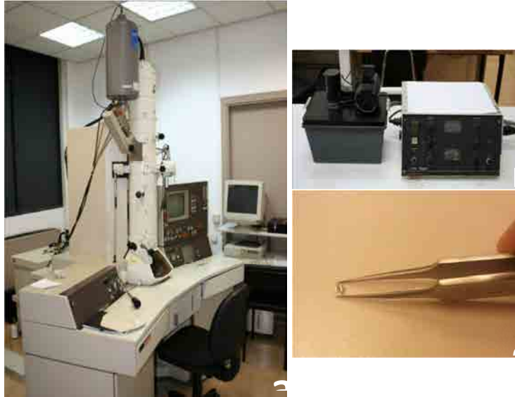
Fig.21 a) Microscope JEOL 1200 EXII used in the assay. b)Electropolishing equipment Tenupol-3 by Struers. c) Sample after the electropolishing ready to be used in the TEM.
