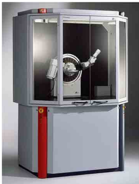
Fig.23 Equipment used in the X-ray diffraction assays. Diffractometer D8 Advance from Bruker.
