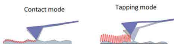
Fig.41 Representation of the contact and tapping mode of the cantilever during surface imaging.
