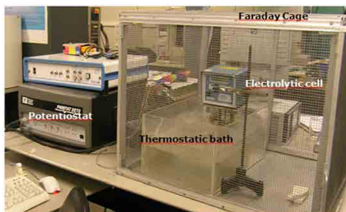
Fig.27 Set up used for the corrosion assays.
