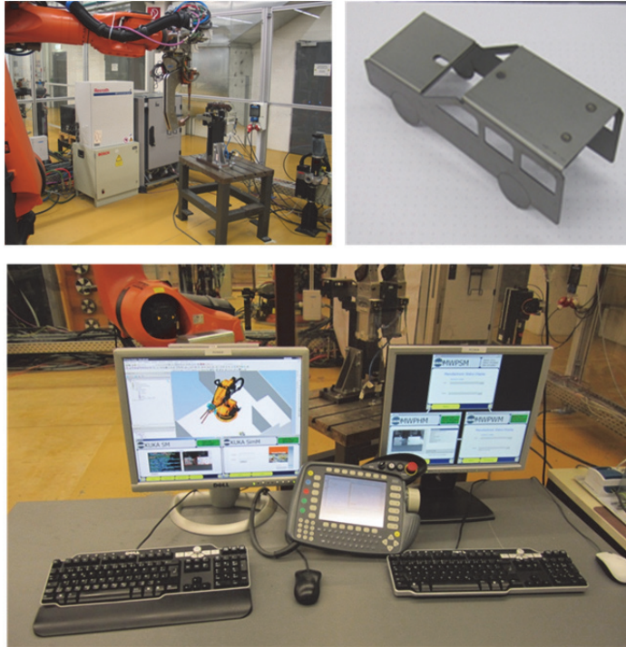
Fig. 51. Setup of the Demonstrator environment in the automotive industry: Typical robot cell (top left), test product (top right) and simulation environment (bottom).
