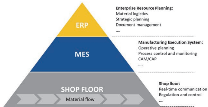
Fig. 16. Traditional automation pyramid with the levels ERP, MES and shop-floor.
