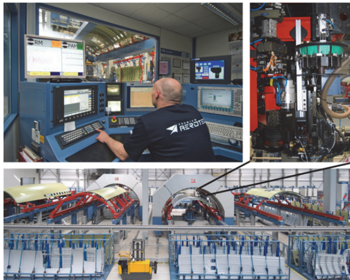
Fig. 49. Working environment in aerospace industry: Operator panel with control systems (top left), riveting head (top right) and factory shop-floor with riveting machines and fuselages (bottom).
