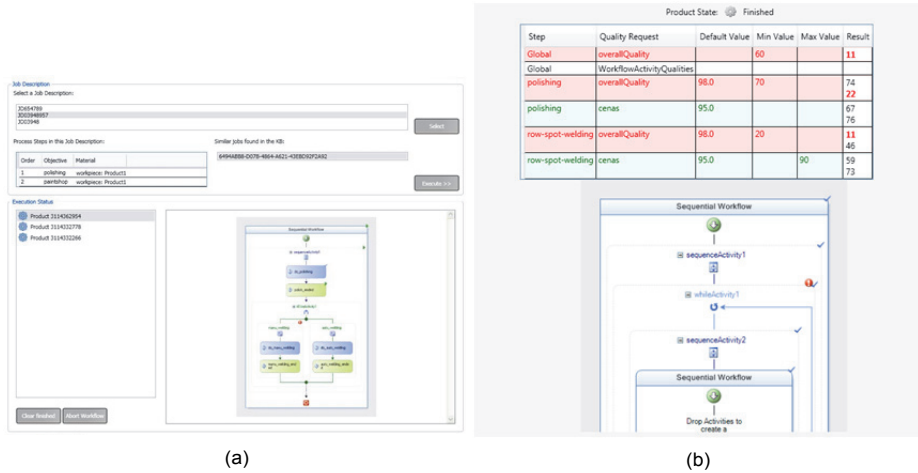
Fig. 45. Graphical user interface for workflow management: (a) Workflow Manager generation on the basis of templates stored in a database; (b) Workflow Manager tracking and process step assessment (Gigler et al. 2012, published by permission of Fraunhofer IPA).
