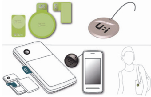
Fig. 10. Concept designs of an RFID accessory for leasing MPDs. Copyright Springer, 2011, Publication IV.
