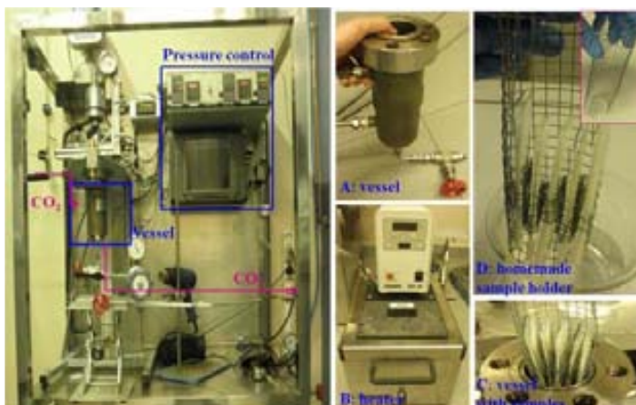
Figure 2.12 The CO 2 supercritical drying system from MATGAS, Spain. A and C) the vessel of SCF 300 mL plant, B) heater, D) our homemade sample holder.
