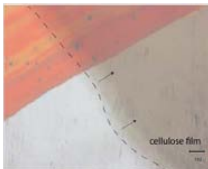
Figure 2.23 Optical image of one sample (BCE-SCD film) immersed in a petri dish with water. The red line on the Petri dish surface is clearly distinguishable through the BCF.
