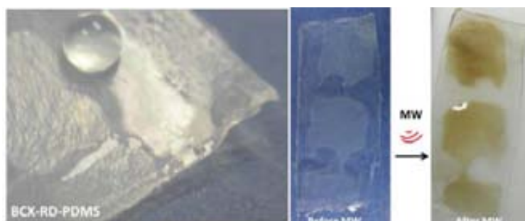
Figure 3.33 BCX-RD-PDMS film, one drop of distilled water on top of the hydrophobic part, which was patterned by PDMS. Then it was cut into rectangular shaped pieces ( \sim 2 \times 1 cm) for MW reaction. After the clean process, iron oxide NPs were observed coating only the hydrophilic parts where there are free -\text{OH} groups.
