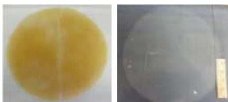
Figure 2.6 A harvested untreated pellicle of GX cellulose (left), compared with the one after clean treatment (right).
