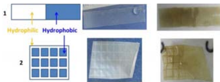
Figure 3.29 First column; Scheme of hydrophobic (blue) and hydrophilic (white) patterns in a BCX-RD-1 film. Second column; BCX-RD-2 film with patterned hydrophobic/hydrophilic zones. A water droplet with large contact angle is displayed in the hydrophobic region. Third column; depicts the patterned BCF-SPIONs composites. It can be seen that darker areas, higher iron oxide load, correspond to the hydrophilic zones of the patterned BCFs.
