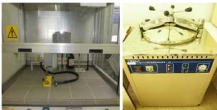
Figure 2.2 Work place in a aseptic hood (left) and the autoclave for sterilization (right).
