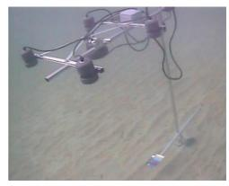
Figure 2.5 The camera system allowed to obtain images from the seabed with same camera angle and distance to the bottom
