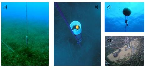
Figure 4.3 Deployment system: a) receiver oriented upwards over seagrass meadows; b) detail of the receiver with the acoustic transductor (in orange); c) sub-surface buoy allocated at 5-8 m depth for ease of the recovery of the system; d) weight mooring ( $\approx$ 20 kg in water).
