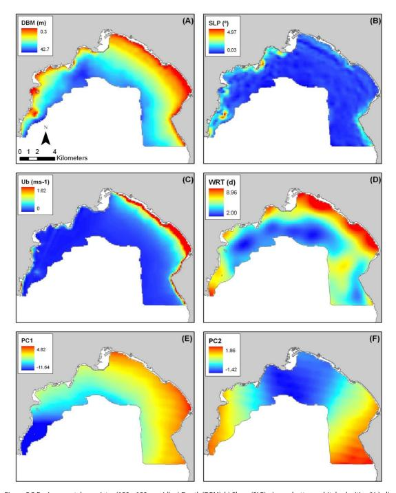
Figure 3.2 Environmental covariates (150 x 150 m grid): a) Depth (DBM), b) Slope (SLP), c) near-bottom orbital velocities ( $U_b$ ), d) water residence time (WRT); e) Landsat PC1, f) Landsat PC2.
