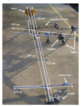
Figure 2.1 Subcam (Albatros Marine Technologies S.L.) system. A video camera is mounted on a metallic structure to obtain standardized images of seagrass cover. The system is dropped from a small boat by an umbilical cable that permits obtaining real-time images.
