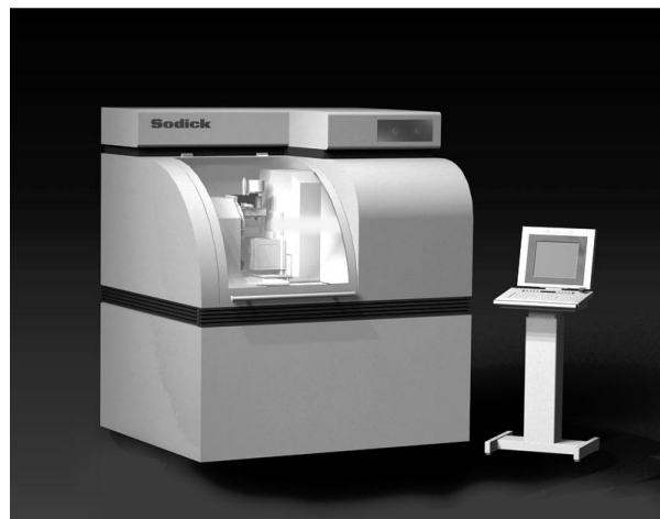
Figure 2.2: Commercial 5-axis control ultraprecision machining centre (Sriyotha et al. 2006).
