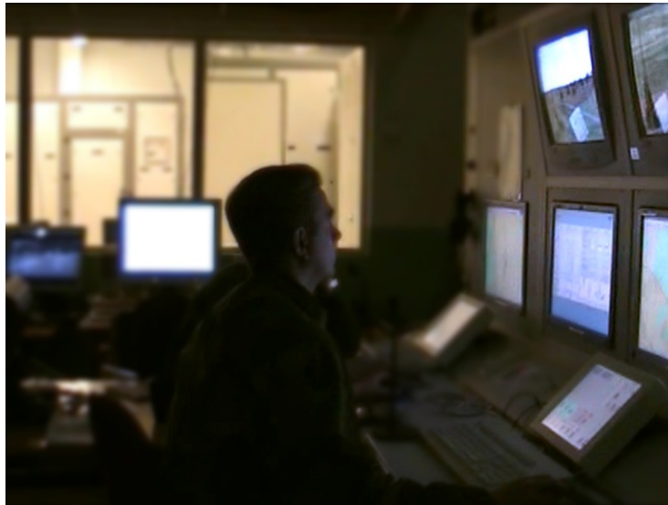
FIGURE 12.2: Instructor station at the SLWC's tank crew training facility (BTA). The top screens display the virtual environment from one of the squad members' perspective or the virtual camera. The bottom screens display the scenario map (left and right screens) and the status information panel (SIP) (middle screen). The small touch screens below the displays control communication.
