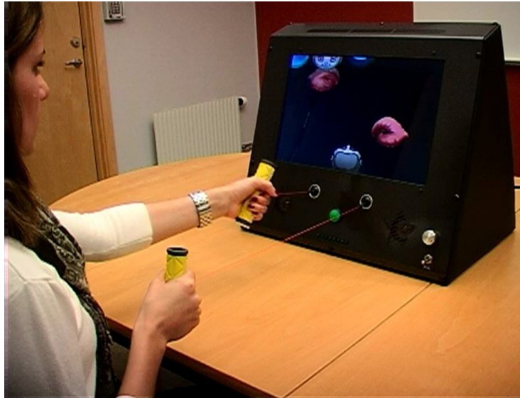
FIGURE 9.1: The Elinor console for stroke rehabilitation in use.
