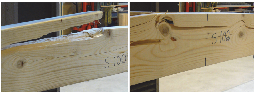
Figure 1. Typical fractures initiated at knots in structural timber subjected to bending load.
