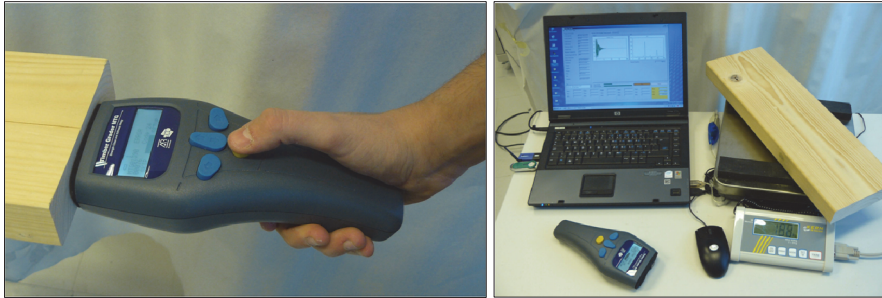
Figure 16. Timber Grader MTG (left) and grading set including grader, balance and computer with applicable software (right).
