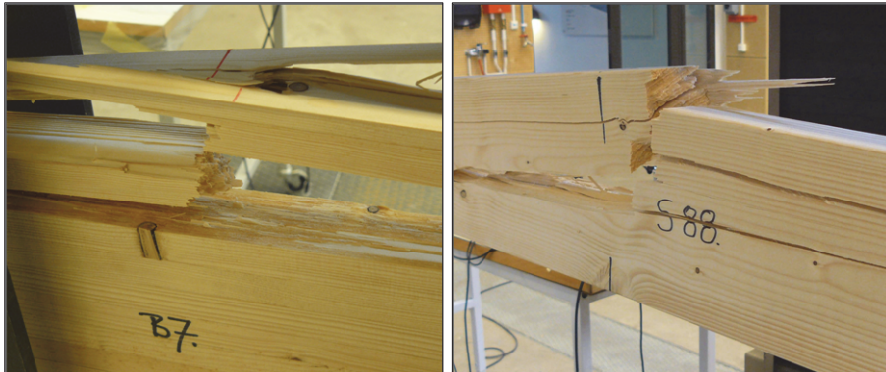
Figure 13. Brittle tensile fractures in compression wood. Left: Lamination fracture in wet glued beam (dim. 50×300×5400 mm) with laminations of Norway spruce side boards. The exhibited beam was tested as part of the research presented in Paper V. Right: Structural timber (dim. 45×145×3600 mm) included in the tests presented in Papers II and III.
