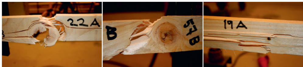
6 Fracture in two of weakest split boards (left and middle) and in strongest split board (right)
