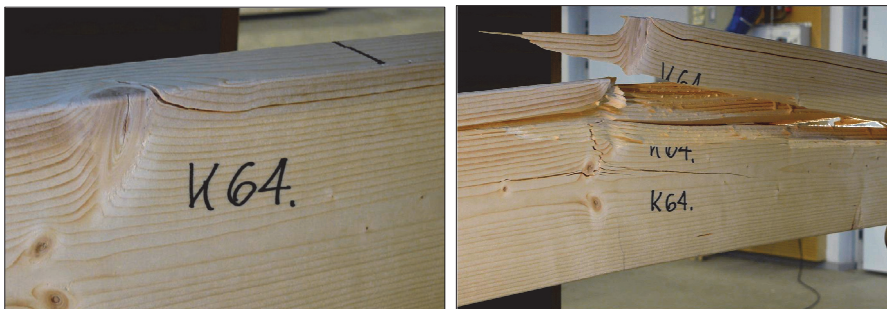
Figure 22. Typical initiation of bending fracture at an outbound arris knot (left) and fully developed fracture (right) in a timber piece of dimension 45 \times 145 \times 3600 mm bent in the upward direction.
