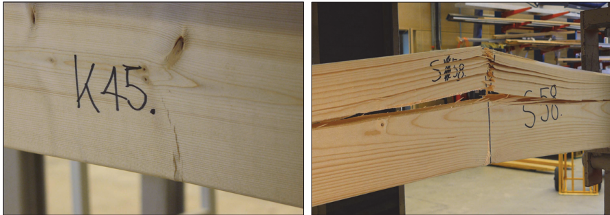
Figure 21. Typical buckling of fibres at compression edge of a board bent in the upward direction (left), and typical subsequent splintered tensile failure (right).
