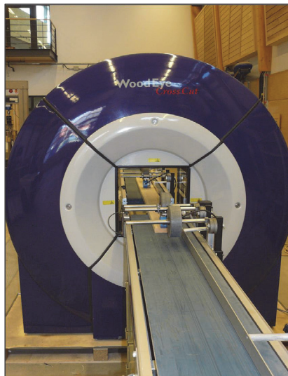
Figure 4. WoodEye scanner of model v4 for optical and laser scanning of timber pieces.
