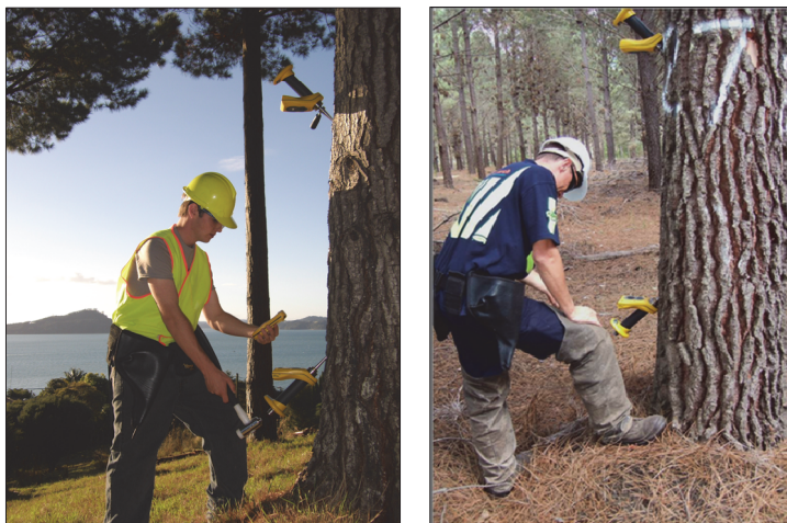
Figure 2. Stiffness property determination on standing trees using acoustic wave velocity measurement. Photos by courtesy of Fibre-gen, Inc., New Zealand.
