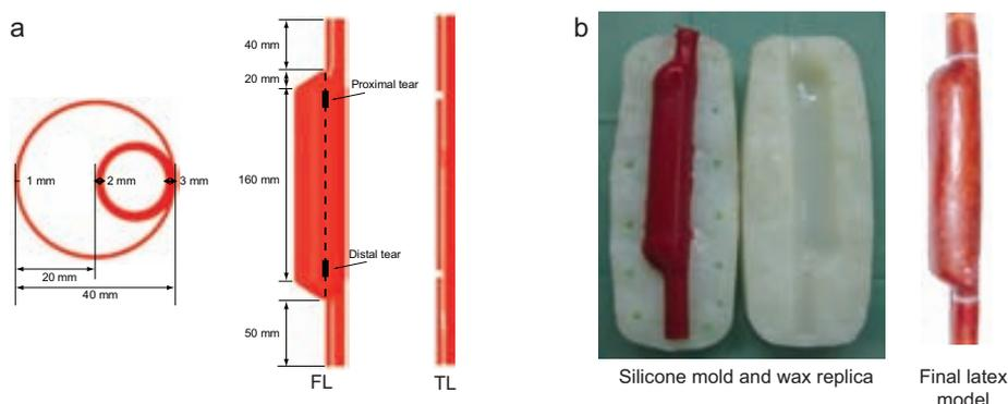
**Figure 3.1:** (a) Synthetic geometry of a type B aortic dissection. Schematic diagram of the dissected aortic section. (b) Consecutive processing steps developed to make latex phantoms of type B aortic dissections.
