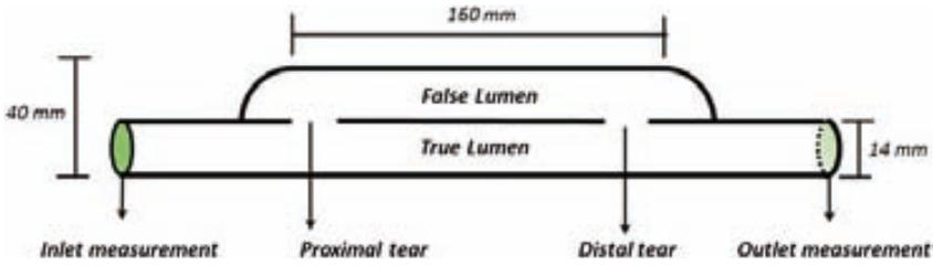
Figure 4.2: Generic geometry of an aortic dissection of type B.
