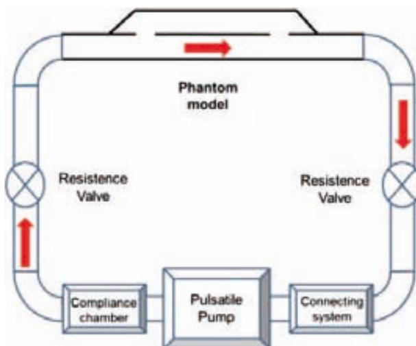
**Figure 4.3:** Schema of the dynamic flow circuit used for the in-vitro experiments.
