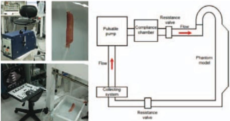
**Figure 2.4:** Experimental set up for the in-vitro measurements. Right: diagram of the circuit. Left: different components of the circuit (top left: pulsatile pump; top right: latex phantom; bottom: portable ultrasound machine and phantom in a water tank).
