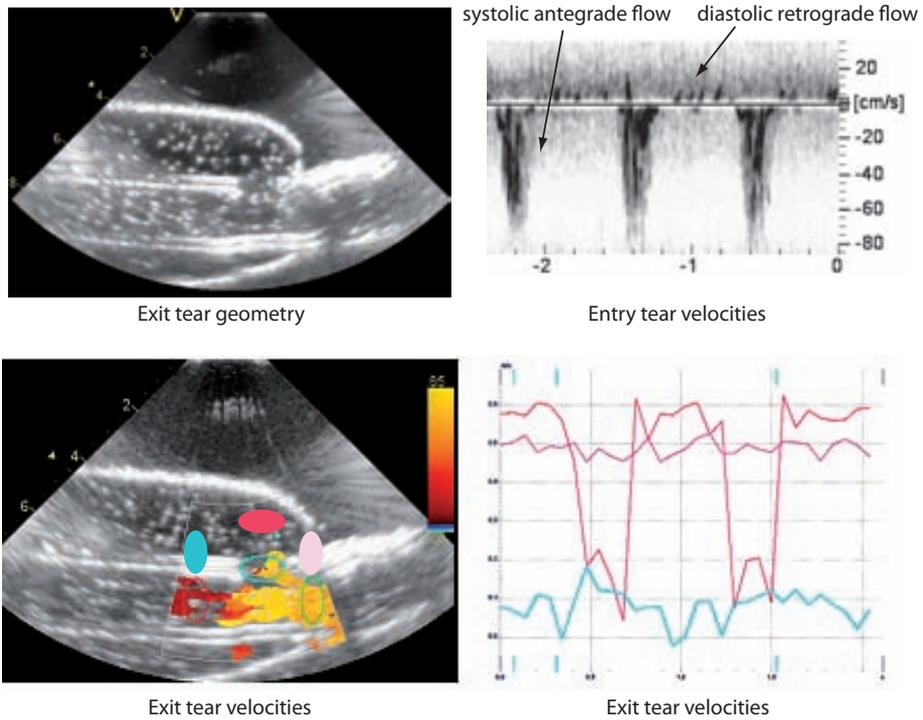
**Figure 2.8:** Echocardiography of the in-vitro setup. Left: longitudinal cut of the phantom at the distal part and colour flow Doppler. Top right: pulsed Doppler velocity waveform at the entry tear; bottom right: colour Doppler velocity waveforms at the exit tear: Red: velocity through the exit tear; Pink: TL velocity distal from the exit tear; Cyan: TL velocity proximal to the exit tear.
