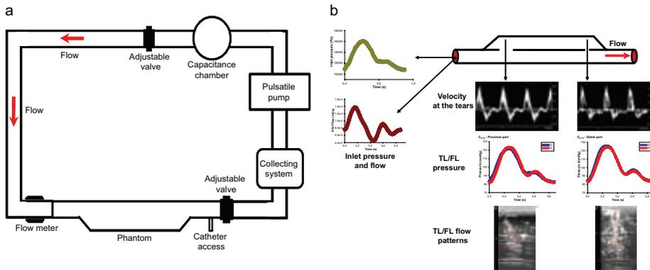
**Figure 3.3:** (a) Diagram of the pulsatile flow circuit. Valves are used to regulate the peripheral resistance and a compliance chamber damps the pump outflow. (b) Example of measurements performed in each model of dissection. *TL*, True lumen; *FL*, False lumen.
