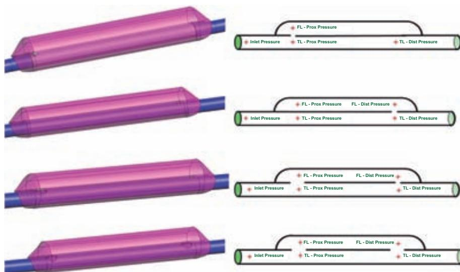
**Figure 4.4:** In-silico FEM geometries (Right) and schematic representation (Left) for the four in-vitro type B AD scenarios. From top to bottom: Case A, Case B, Case C and Case D.
