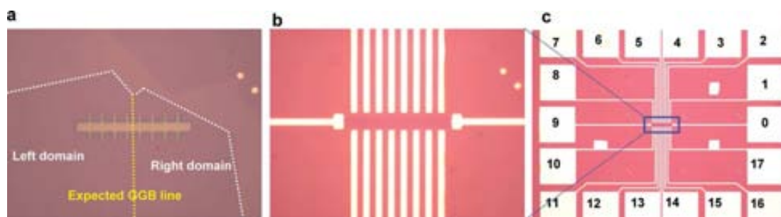
Figure 4.21: Optical image of the four-probe device across a GGB. a) E-beam lithography resist (PMMA) location at a merging region including a GGB. b)-c) A final device with Hall bar geometry at merging region of two graphene domains.
