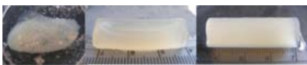
Fig. 3 Physical appearance of different pectin gel monoliths after solvent exchange to ethanol: HM-pectin from citrus with (left) and without (middle) sucrose addition during gelation, and HM-pectin from apple-citrus without sucrose addition (right).
