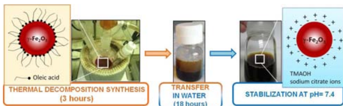
Figure 1. Schematic description of the thermal decomposition process used for TD-SPIONs synthesis. The first step is the formation of magnetic material in the high temperature boiling solvent, in presence of organic surfactants. The second step is the ligand exchange with the anionic surfactant TMAOH which takes place during 18 h. In the last step there is the separation and stabilization at pH=7.4 of the colloidal aqueous phase.
