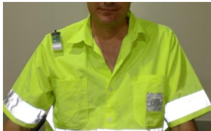
Figure 4.2.3 HOBO data logger used for personal light monitoring placed at the shoulder level.
