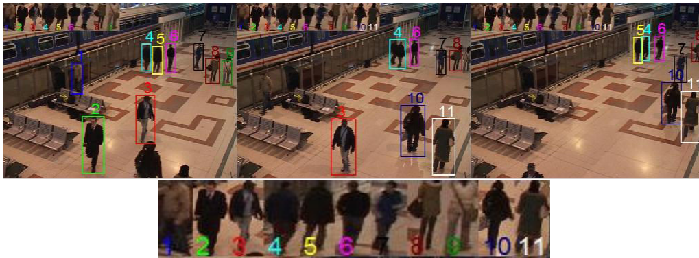
Figure 7.5: Tracking results for PETS'06. The bottom displays 11 objects that we initialize and track successfully. Our results have no identity switch or incorrect novel object initialization.
