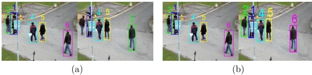
Figure 7.1: Tracking results only with color feature (a) and with feature integrating color and 2-dimensional coordinates (b). In (a), object 6 switches into object 2 after 13 frames due to similar appearance.
