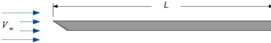
Figure 2.15: Flat plate aligned with the flow approaching.
