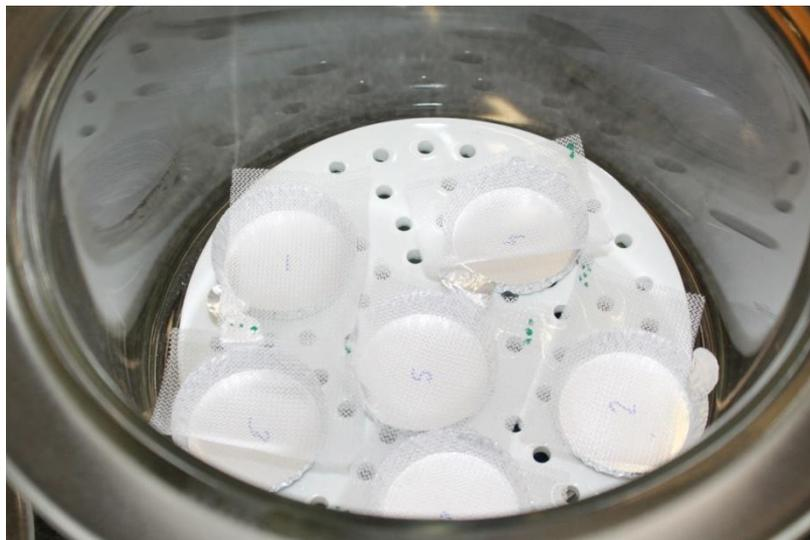
Figure 31: Storage of PP fabrics in a desiccator to avoid humidity absorption.
