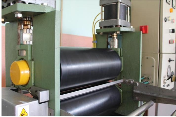
**Figure 38: Padding equipment used for homogenization of the active principle on the PA or PP sample after impregnation process.**
