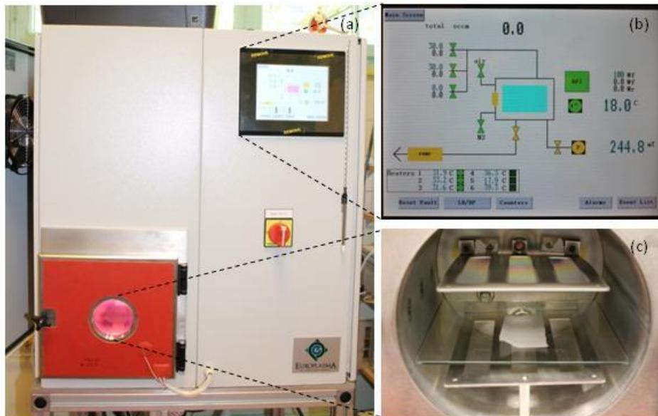
**Figure 34:** Europlasma Junior Advanced PLC low-pressure plasma equipment using with air as gas for plasma generation (a). Focus of the panel control screen (b) and the inside of the chamber (c).
