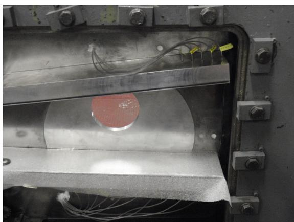
**Figure 2.12:** *The two ramps instrumented for the qualification test campaign: the upper ramp features five pressure taps, the lower ramp ten*
