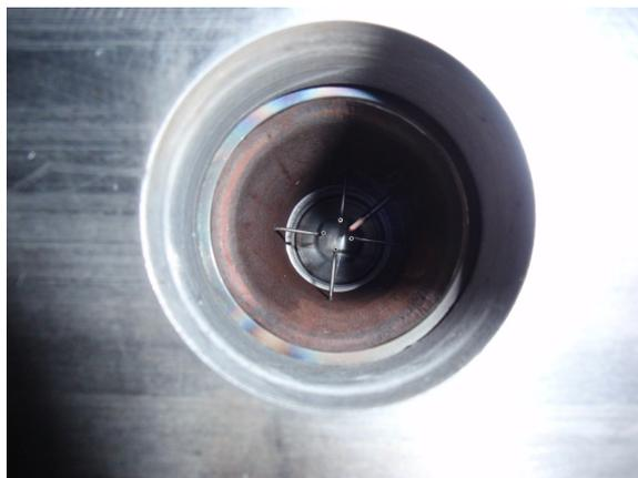
**Figure 2.11:** *The front view of the four static pressure L-shaped taps and the thermocouple that instrument each of the aspiration system four tubes*
