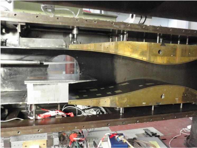
**Figure 4.17:** *The test section with the shock generator, and the convergent-divergent 2-D nozzle for Mach 2*
