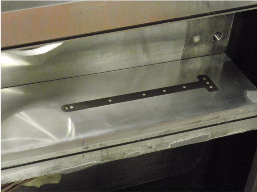
**Figure 3.2:** *The PCBs insert on the bottom ramp of the supersonic wind tunnel divergent*
