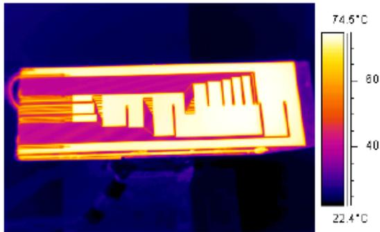
**Figure 3.7:** *Infrared image of the thin-films insert top heated up by Joule heaters glued on its bottom*
