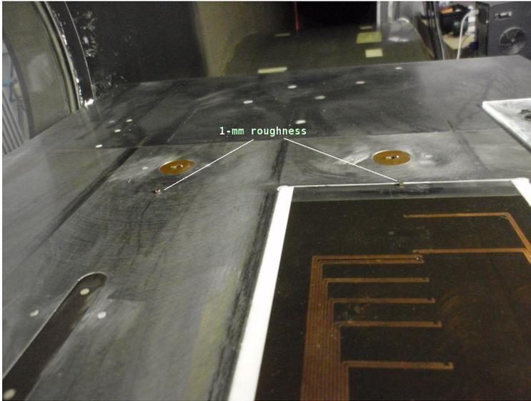
**Figure 4.19:** *Zoomed view on the two instrumented inserts on the plate: each of them has a dedicated electrodes plug or roughness*
