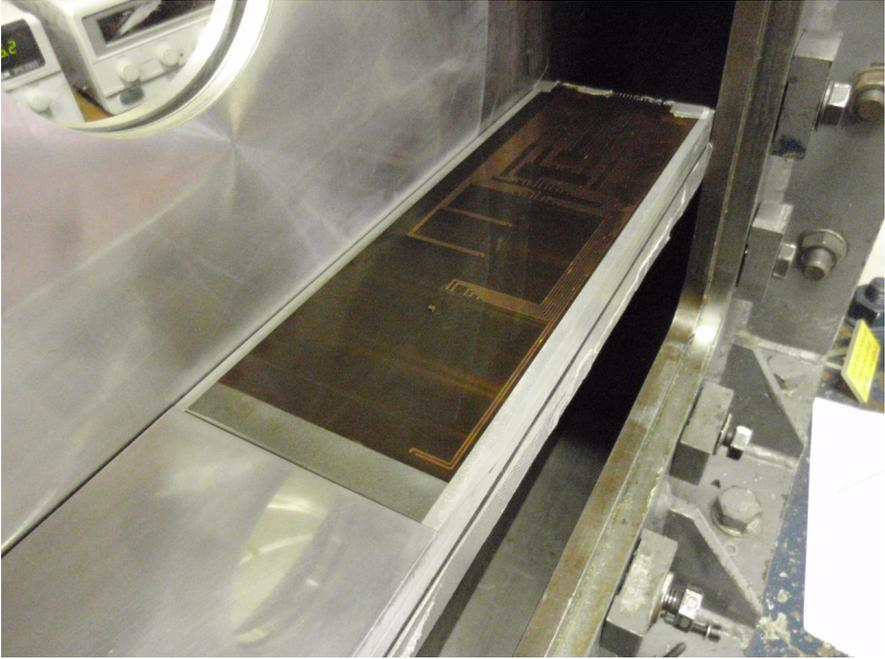
**Figure 3.1:** *The thin-films insert on the bottom ramp of the supersonic wind tunnel divergent*
