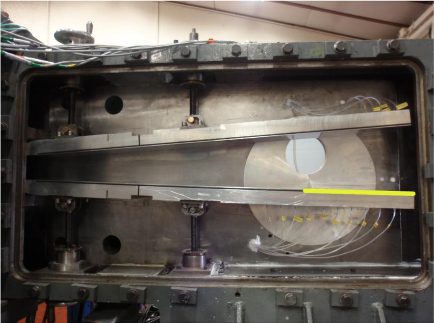
**Figure 3.3:** *General view of the supersonic wind tunnel divergent with the inserts location highlighted*
