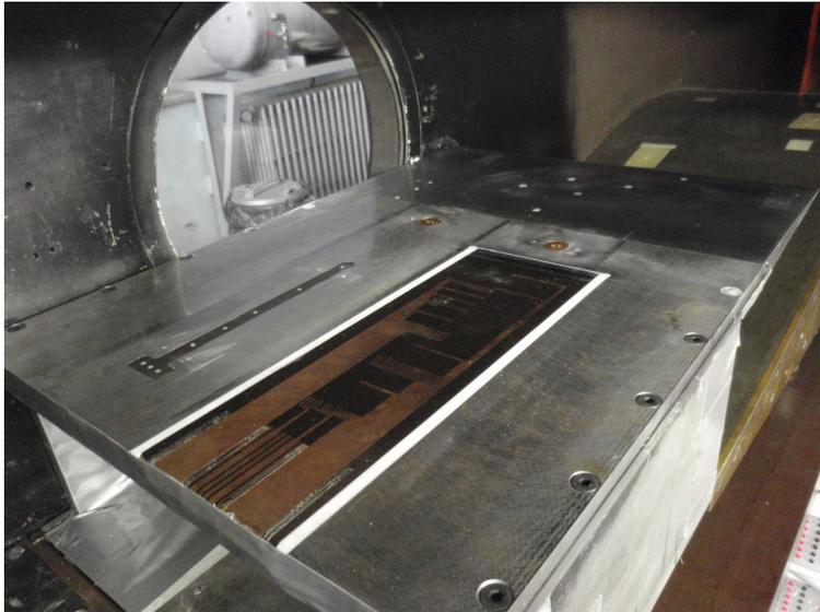
**Figure 4.18:** *The layout of the two instrumented inserts on the plate (the PCBs insert is on the left, the thin-films insert is on the right)*
