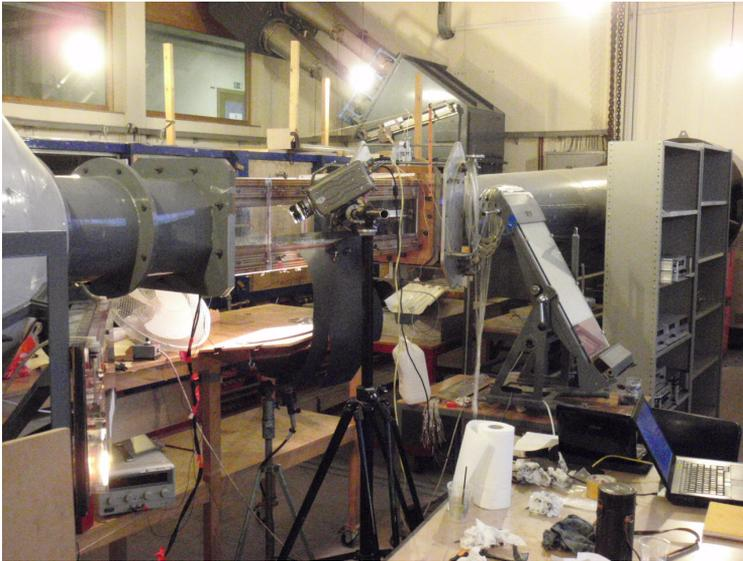
**Figure 4.6:** *A view of the low-speed wind-tunnel with the set up for smoke-sheet visualizations*
