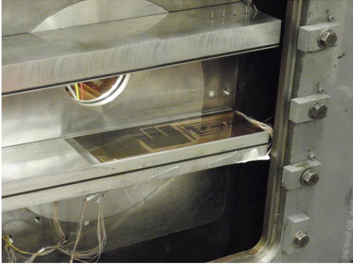
**Figure 3.6:** *The thin-films insert embedded in the lower ramp of the supersonic wind tunnel*
