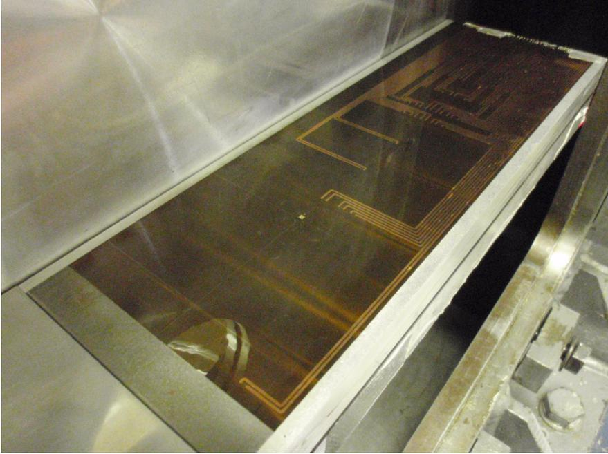
**Figure 3.18:** *The thin-films insert into the lower ramp of the supersonic wind tunnel*
