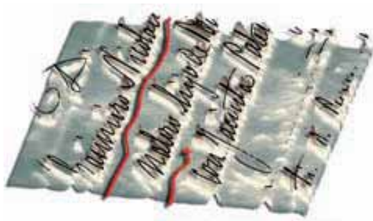
Figure 3.2: In a 3D-view, text lines can be seen as peaks and the space between them as valleys.
