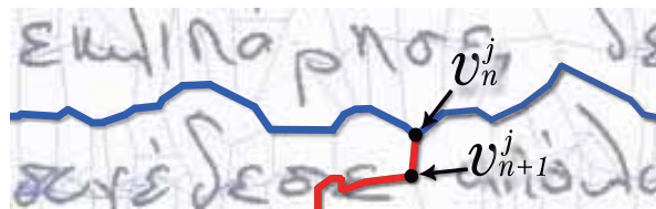
(c) Back Heuristic. The blue line represents the correct path computed. Red line is a wrong possible path going back.
