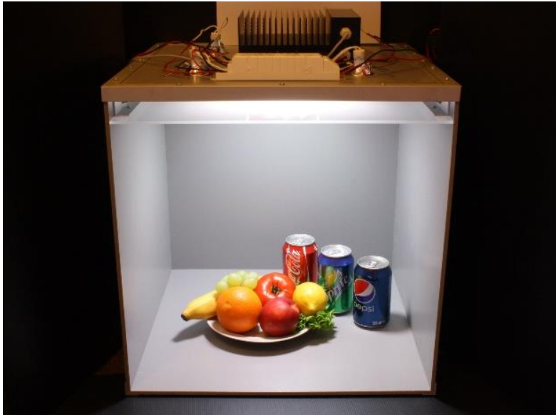
Fig. 2.3. Experimental cabinet with the tuneable RAGB source mounted on top and illuminated objects placed inside [P5].
