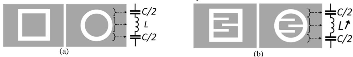
Figure 81 Problematic of meandered patch antennas. (a) regular patch antenna at the aperture of the cavity. (b) meandered patch antenna at the aperture and the model havin increased inductance compared to the regular case.
