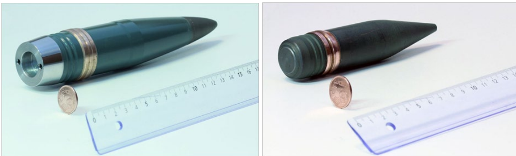
Figure 112 (a) 40 mm caliber projectile with a drilled cavity of 20 mm in diameter. (b) 30 mm caliber projectile into which a 16 mm diameter cavity can be drilled.
