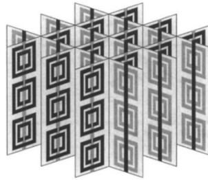
Figure 50 Depiction of the wire-SRR metamaterial of Shelby et al. used to verify negative refraction. The sample was irradiated by a microwave beam at 10.5 GHz incident at 18.43^\circ , and a microwave detector was scanned azimuthally around the exit point in the plane of incidence. A control sample made of Teflon reported a positive angle of refraction of 27^\circ , corresponding to the well-known refractive index of Teflon of + 1.4, and calibrating the apparatus. Using the wire/SRR metamaterial, the same beam was observed to exit at an angle of -61^\circ , which, applied to Snell's Law, yields an effectively negative index of refraction of -2.7.
