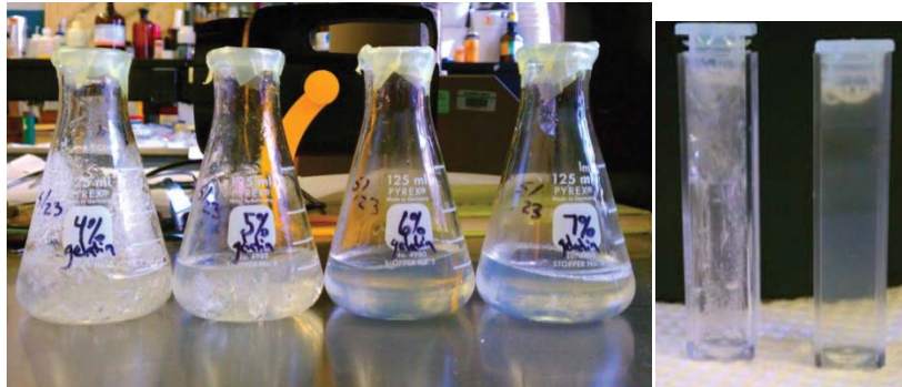
Figure 10. Left, illustration of effects of low temperature (5°C) storage, 4% and 5% gelatin by weight exhibited freeze fracturing. Right, individual cuvettes illustrating freeze fractured and intact samples.
